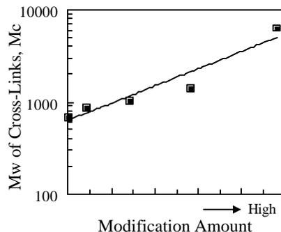
Figure 3 - Molecular Weight of Cross-Links ( $M_c$ )
