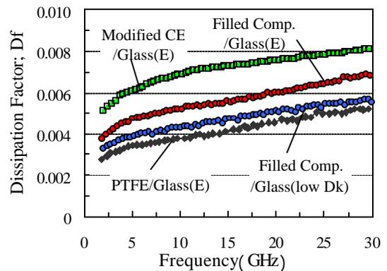
**Figure 10 - Dissipation Factor up to 30GHz**
