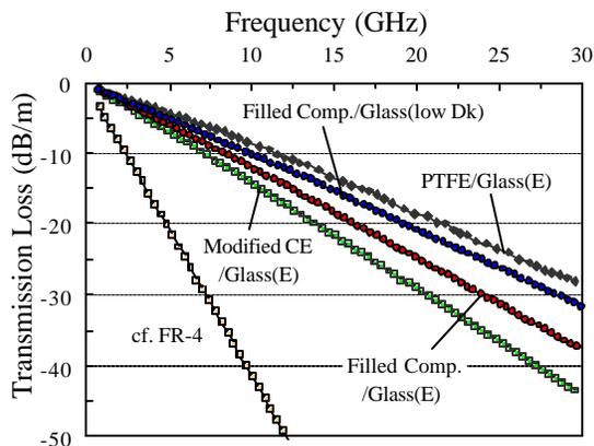
**Figure 9 - Transmission Loss up to 30GHz**
