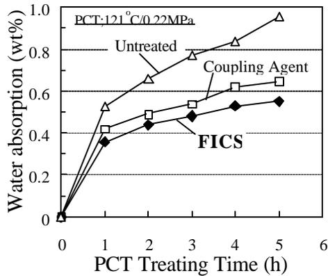
Figure 7 - Water Absorption of Resin with Filler
