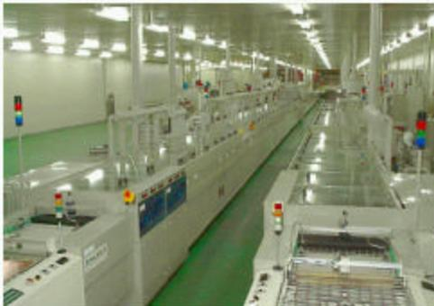
**Figure 38 - 2 Fully Integrated Lines: Debur / Desmear / Electroless**
