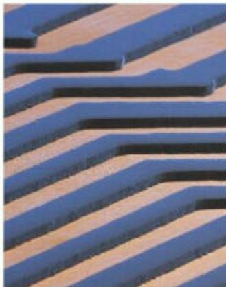
**Figure 28 - SEM Lines 40 μm - Very Straight Sidewalls**
