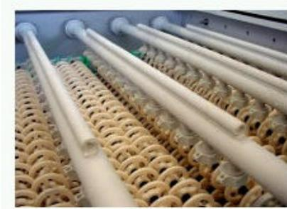
**Figure 7 - Cascading Rinse with Spray Bars**
