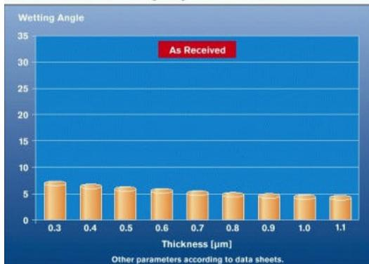
**Figure 9 – Wetting Angles for As Received Solder Paste**
