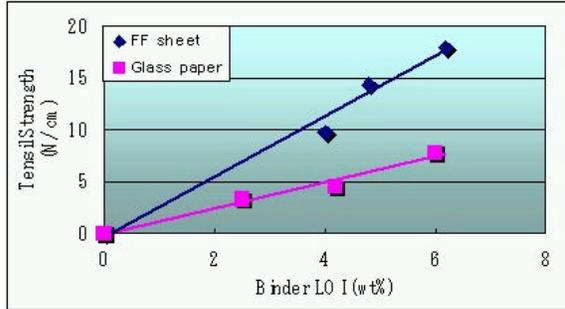
**Figure 15 – Comparison of Base Material Strength Between FF Sheet and Glass Paper on 20g/m<sup>2</sup> Base Material**
