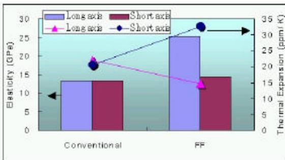
**Figure 3 - Effects of Glass Fiber Shape on Laminate Elasticity and Thermal Expansion at Same Cross-Section Area Fibers**
