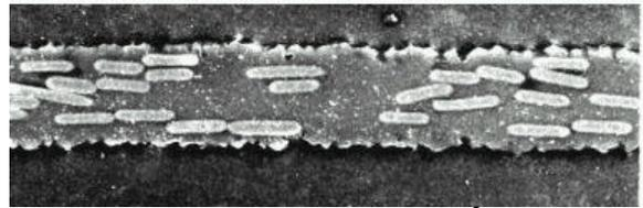
**Figure 7 – Cross-Section of  $13\text{g}/\text{m}^2$  FF Sheet Laminate**
