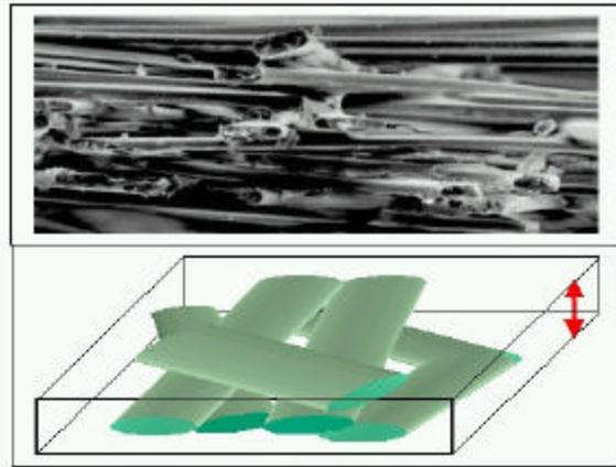
**Figure 6 – Cross-Section Photo and Image Scheme of FF Sheet**
