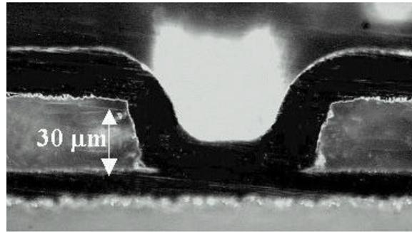
**Figure 13 - Finished Condition of Laser Processing on 30 mm Type FF Sheet Laminate Laser= 10mJ – 1Shot**
