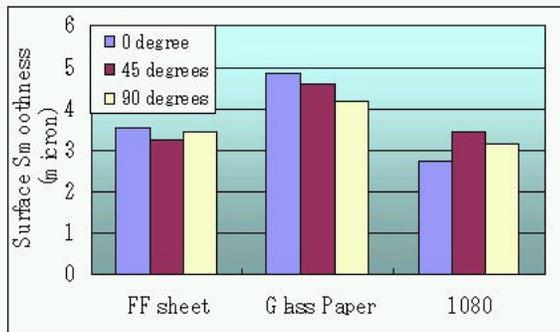
**Figure 12 - Surface Smoothness Comparison of FF Sheet, Glass Paper and 1080 Type Cloth for Three**
