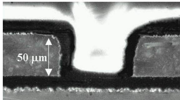
**Figure 14 - Finished Condition of Laser Processing on 50 mm Type FF Sheet Laminate Laser= 10mJ – 1Shot**
