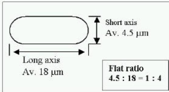
**Figure 2 – Cross-Section Scheme of FF**
