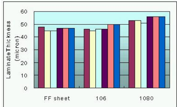
**Figure 8 - Comparison of Laminate Thickness Among Six Points in A Laminate**
