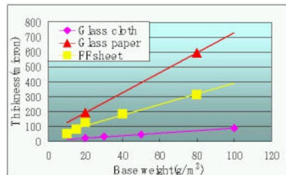
**Figure 4 - Material Thickness vs. Base Weight of Glass Cloth, Glass Paper and FF Sheet**
