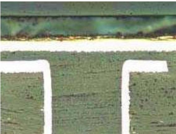
**Figure 16 - Cross-section of IVH Core: Glass cloth (t=0.2 mm) Hole = 0.2mm Buildup: 13g/m<sup>2</sup> FF sheet (t=0.03mm)**
