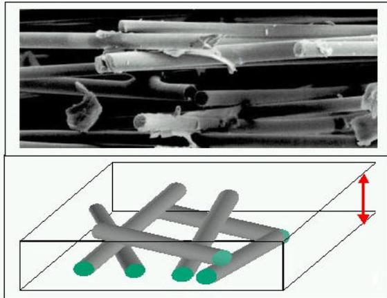
**Figure 5 – Cross-Section Photo and Image Scheme of Glass Paper**
