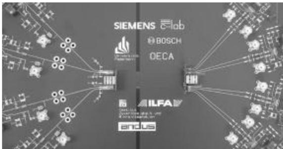
**Figure 22 – Printed Circuit Board with an Entire Electrical-Optical Interconnection**
