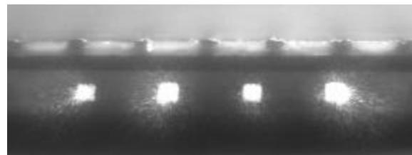
**Figure 18 – Cross section of a multiplayer printed circuit board with integrated optical waveguides, illuminated with VCSELs**
