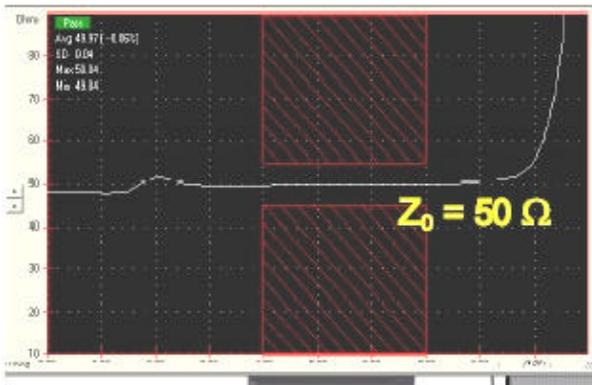
**Figure 1 - Typical TDR from a Production Environment<sup>2</sup>**
