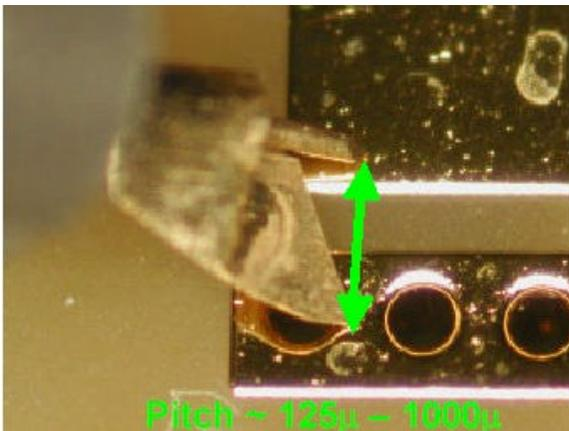
**Figure 2 - Close up of Precision Microprobes with Very Small Parasitics and Capable of being Calibrated Right to the Tip**
