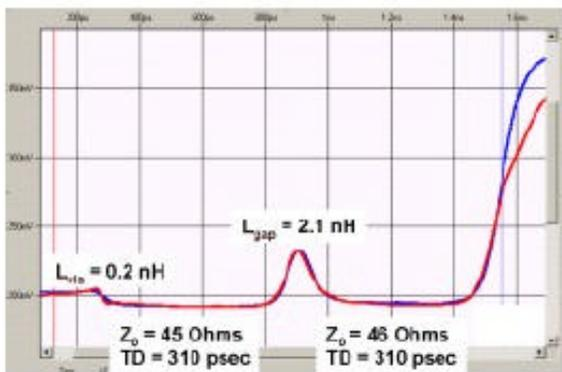
**Figure 7 - Comparing the Measured and Simulated TDR Profile for this Transmission Line with a Gap in the Return Path<sup>6</sup>**
