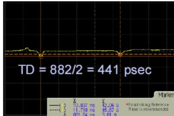
**Figure 3 - Profile from a Trace with Two Small Squares Spaced 3 Inches Apary - From the Precision TD Measurement, the Velocity of a Signal can be Accurately Measured<sup>3</sup>**
