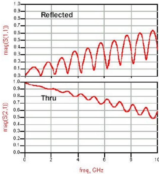
**Figure 4 - Measured S11 and S21 of a 3 Inch Long Stripline Only the Magnitude of the S Parameters is Shown Here<sup>4</sup>**
