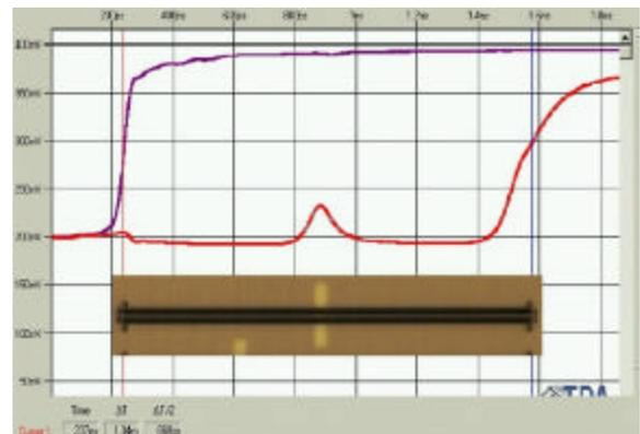
**Figure 6 - Measured TDR Profile of a Transmission Line with Initial Via and Small Gap in the Return Path**
