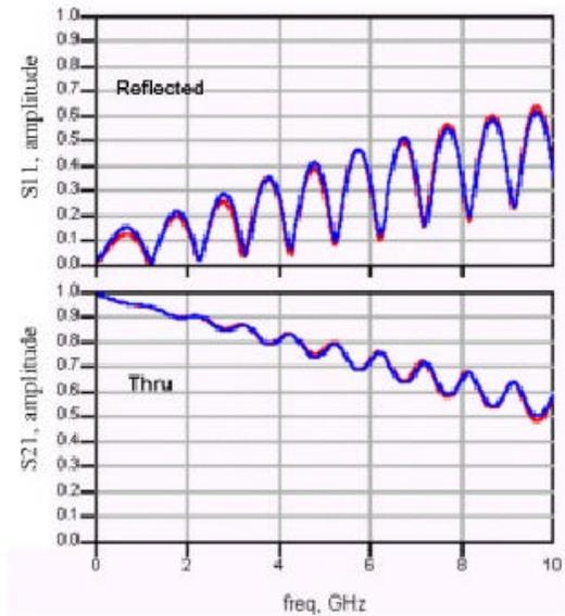
**Figure 5 - Comparison of the Measured and Simulated S Parameters for the 3 inch Transmission Line<sup>5</sup>**
