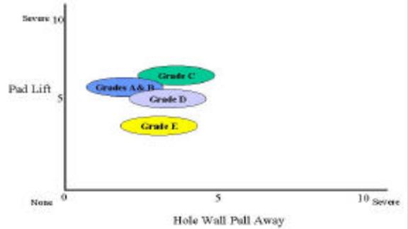
**Figure 5 - 6X Solder Float Performance By Grade .040\"/>**
