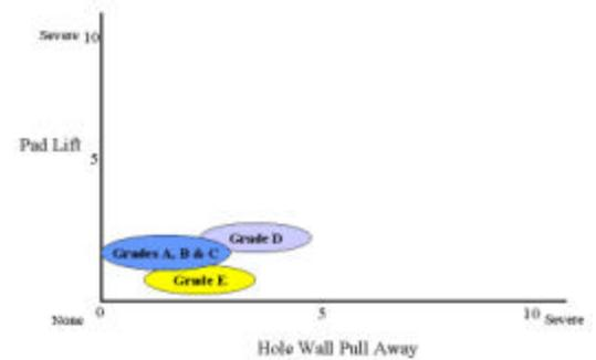
**Figure 7 - 6X Solder Float Performance By Grade .0135\"/>**
