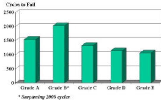
Figure 1 – IST Performance Ambient to 150 °C (Cycles to Fail for Barrel Cracking)
