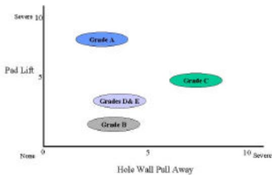
**Figure 4 - 6X Solder Float Performance By Grade .040\"/>**
