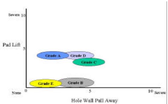
**Figure 6 - 6X Solder Float Performance By Grade .0135\"/>**
