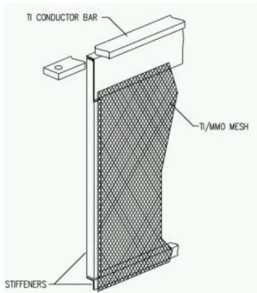
**Figure 4 – Typical Titanium/MMO Structure Used For Plating Operations**
