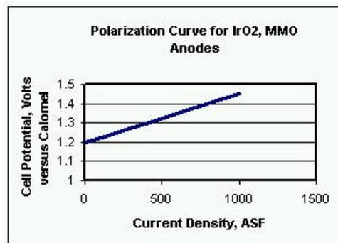
**Figure 3 – Anode Potential vs. Current Density**
