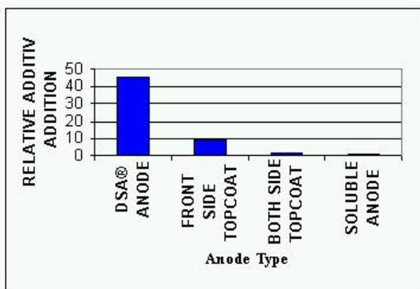
**Figure 7 – Oxidation of Commercial Brightening and Leveling Agents Anode and Typical Insoluble Anodes Compared with Soluble Anodes**
