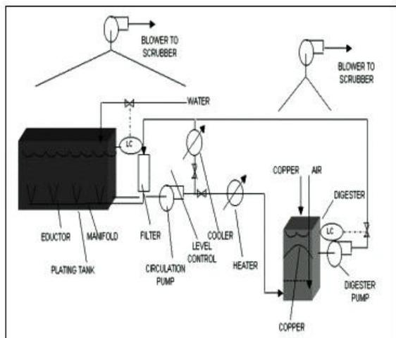
**Figure 5 – Flow Diagram of a Copper Digester for Use with Insoluble Anodes**
