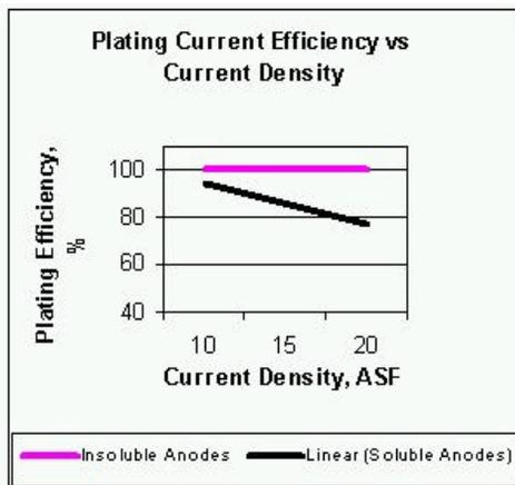
Figure 8 – Current Density Versus Plating Efficiency
