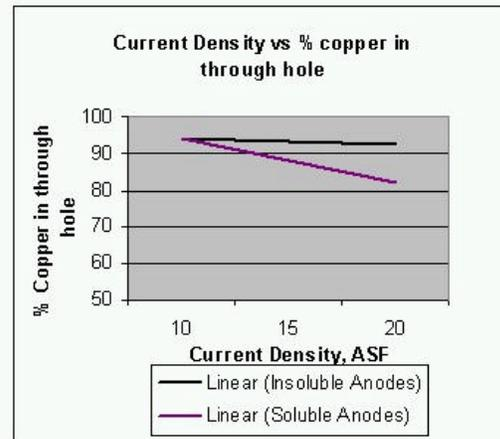
Figure 9 – Current Density Versus Ratio Of Copper In The Through Hole
