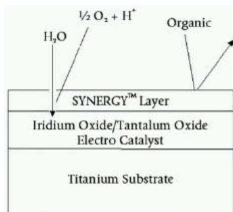
**Figure 6 – Addition Agent Protection Using Proprietary Coating System**
