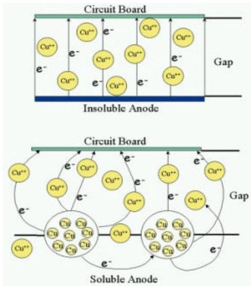
**Figure 1 – Current Distribution: Continuous Planar Anodes vs. Typical Soluble Anodes**
