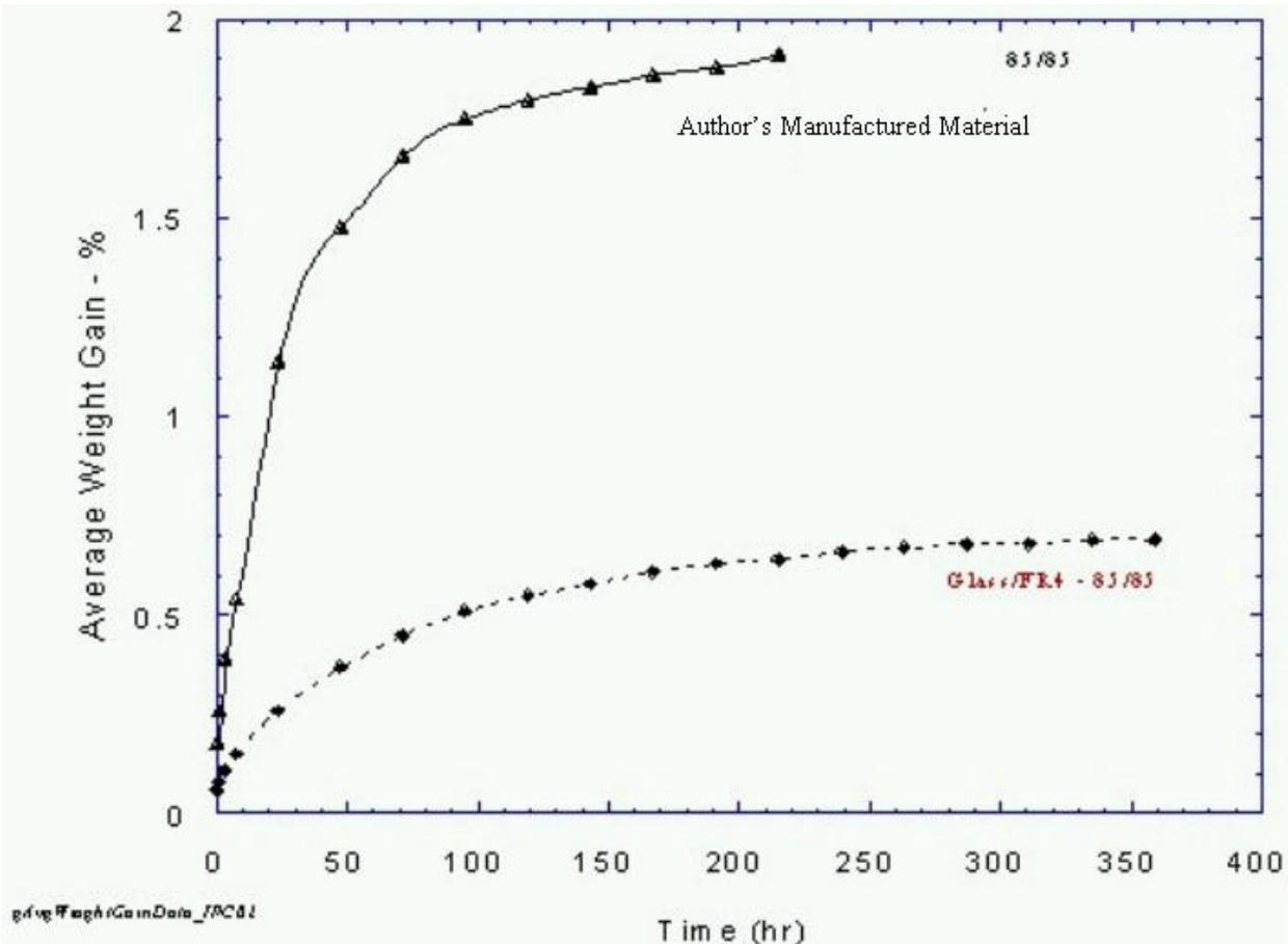
**Figure 1 - Rate of Moisture Absorption of PWB Laminates With Aramid Paper (3N710/Epoxy - 47/53 - 0.06" Thick)**
