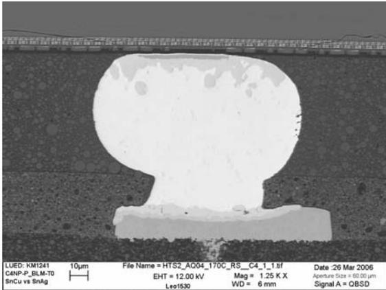
Figure 9a - HTS 170C/1000hrs Sn2.0Ag C4
