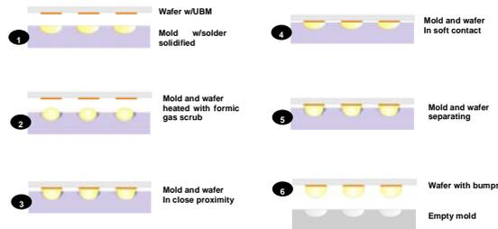
**Figure 3 - Solder transfer process sequence.**
