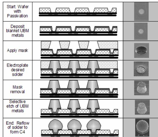
**Figure 4 - Electroplated C4 Process Flow**
