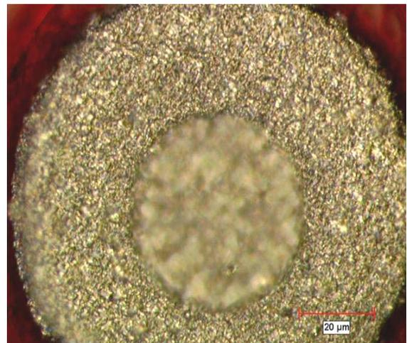
**Figure 7 - Rupture in UBM in Lead-Free**
