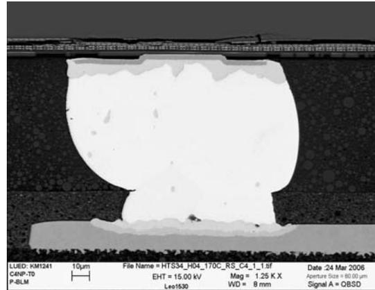
Figure 9b - HTS 170C/1000hrs Sn0.7Cu C4
