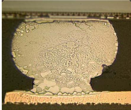
**Figure 8a - X-section of PbSn C4 post DTC**
