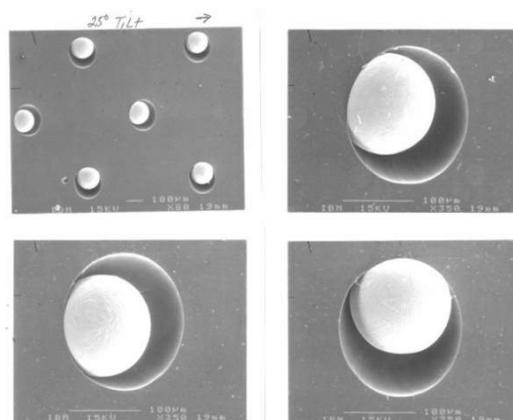
Figure 2 - Reflowed solder spheres in glass mold cavities prior to transfer to wafer.
