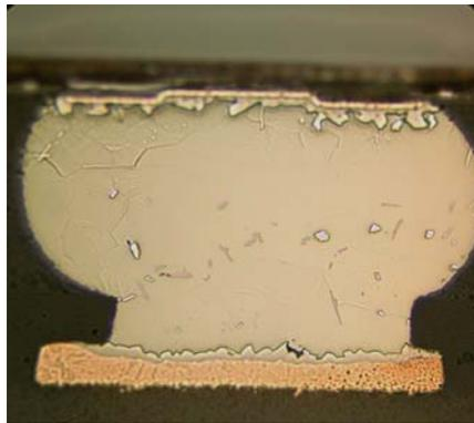
**Figure 8b - X-section of SnAg C4 post DTC**
