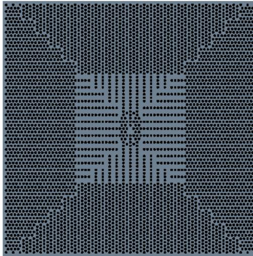
**Figure 5 - 200 um pitch test vehicle C4 pattern.**
