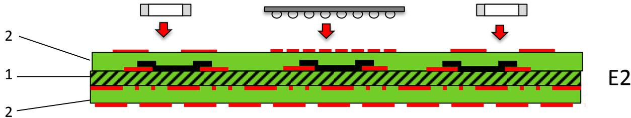
Mounting base example with formed passive components inside the mounting base turning the product into an base-core ready for component mounting to complete an Embedded Component Board Assembly
