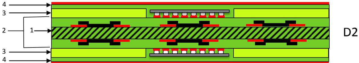
*Base-core example with formed passive components in the mounting base and inserted active components on both sides*
