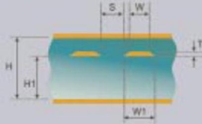
Coated Coplanar Waveguide With Ground
