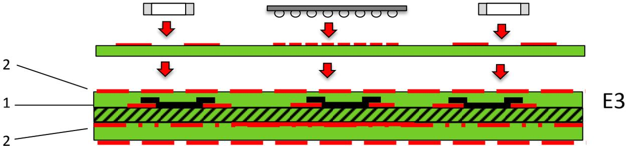
Mounting base example with formed passive components inside the mounting base plus additional layering added to one or both sides to complete the Embedded Component Printed Board ready for component mounting to complete an Embedded Component Board Assembly
