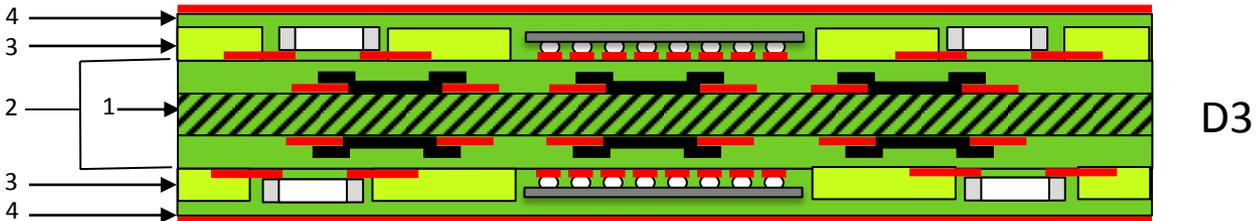
*Base-core example with formed passive components in the mounting base and inserted passive and active components on both sides*
