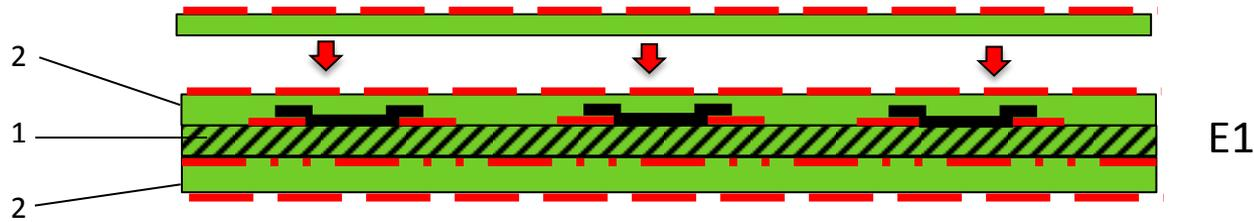
Mounting base example with formed passive components inside the mounting base plus additional layering added to one or both sides to complete the Embedded Component Printed Board
