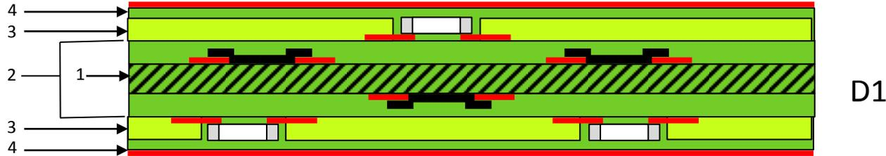
*Base-core example with formed passive components in the mounting base and inserted passive components on both sides*
