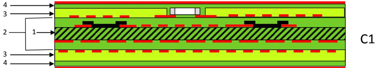
*Base-core example with formed passive components in the mounting base and inserted passive components on one side*
