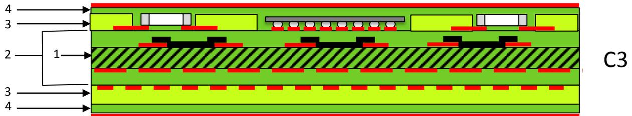
*Base-core example with formed passive components in the mounting base and inserted passive and active components on one side*
