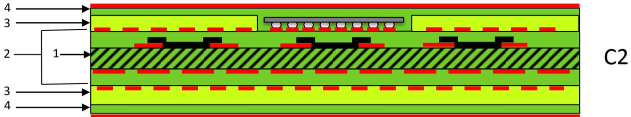
*Base-core example with formed passive components in the mounting base and inserted active components on one side*
