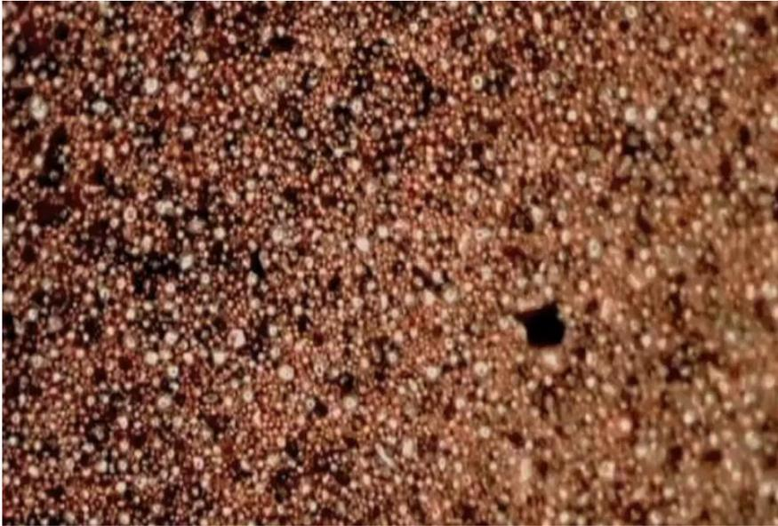
Copper and alloy particles in a liquid organic formulation
