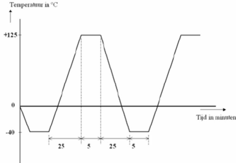
**Figure 1 - Schematic of the Thermal Cycling Tests (TCT)**
