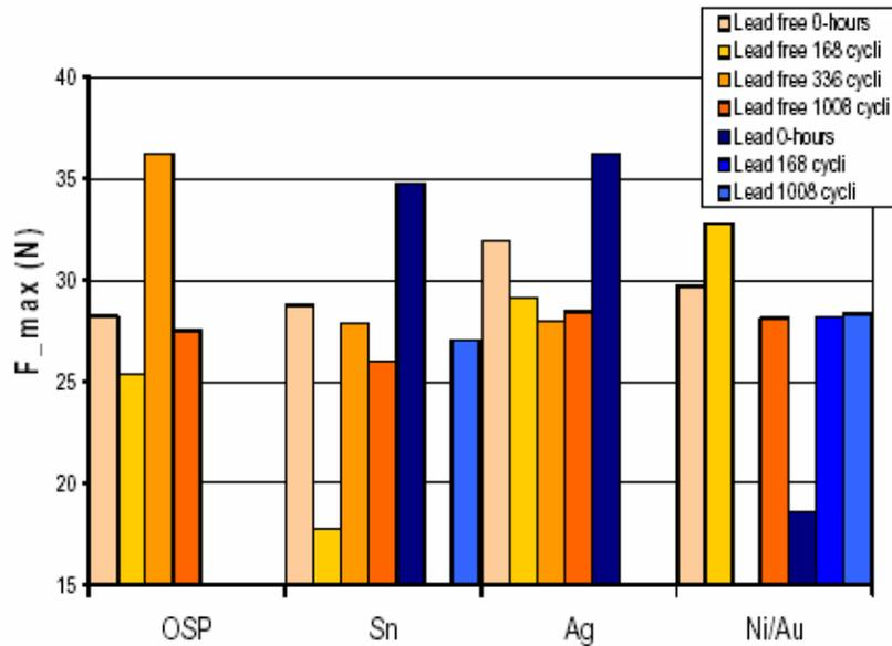
**Figure 10 - Tensile strength test results: The maximum force on the corner lead of the S016 component grouped by board finish and displayed for the lead-free and lead containing joints, after a specified number of TCT-cycles.**
