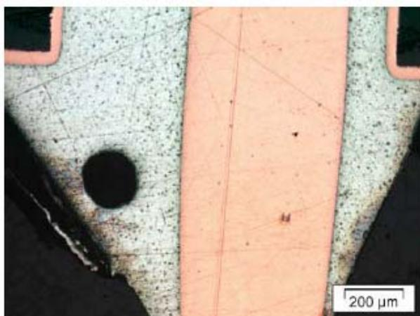
**Figure 4 -PTH Component before TCT for SnPb Solder**
