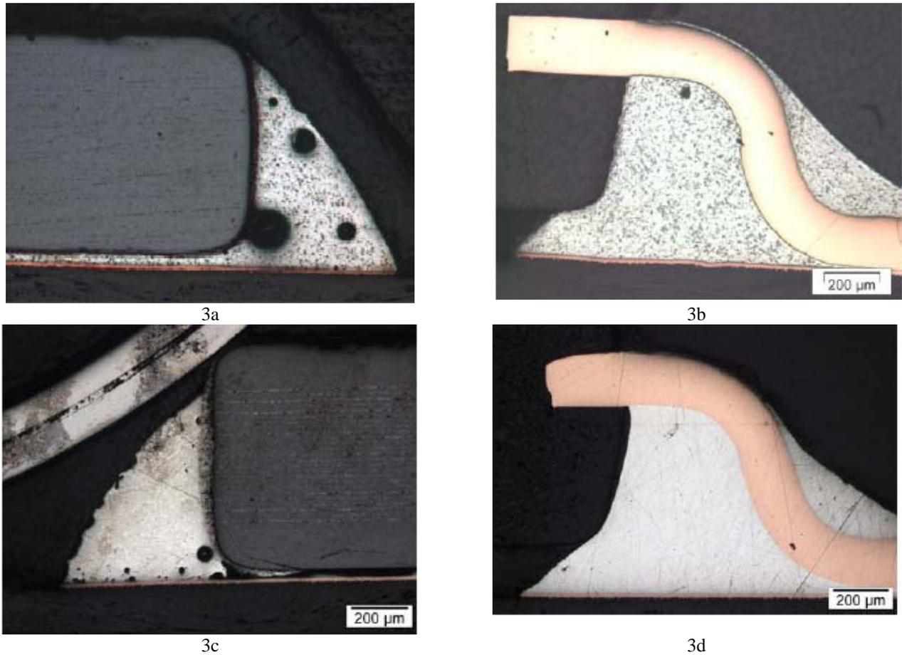
**Figure 3 - SMD Components before TCT for a) SnPb (solder), Sn- (Board)Finish, SOT (Component); b) SnPb, Snfinish, Capacitor; c) SAC, Ag-Finish, Capacitor; d) SAC, Aufinish, SOT**
