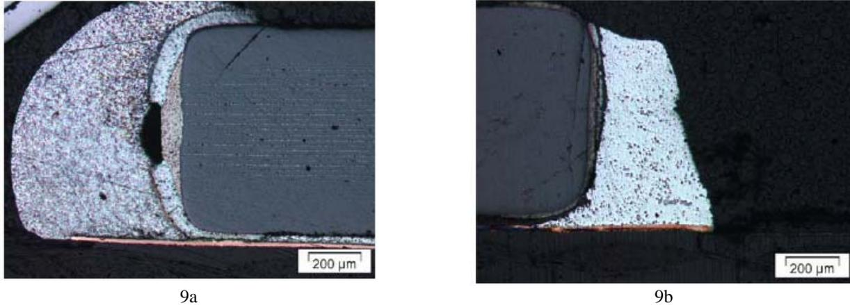
**Figure 9 - a) lead containing solder, Ag board finish, capacitor, b) lead-free solder, Ag board finish, capacitor**
