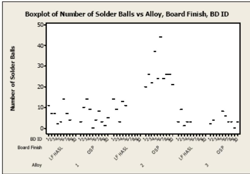
Figure 11 - Confirmation Run Box Plot for Solder Balls
