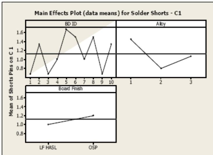
Figure 17 - Confirmation Run Main Effect Plots for Solder Shorts
