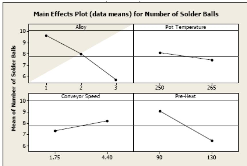
Figure 8 - DOE Main Effect Plots (data means) for Solder Balls
