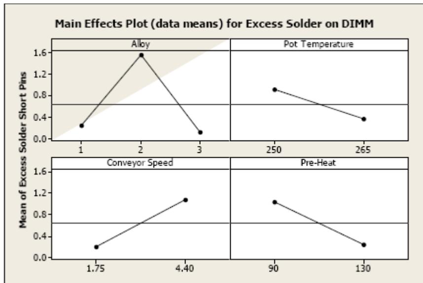
Figure 19 – DOE Main Effect Plots (data means) for Excess Solder
