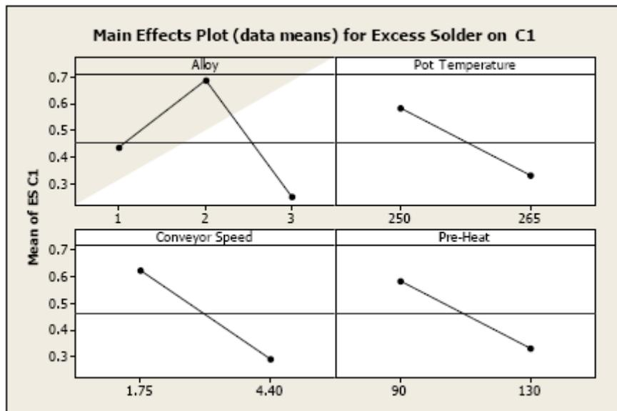
Figure 20 - DOE Main Effect Plots (data means) for Excess Solder
