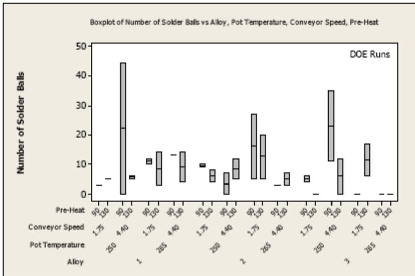
Figure 10 – DOE Box for Solder Balls
