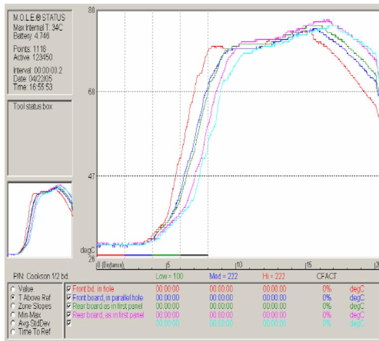
**Figure 3 – Rapid and Uniform Affect on the board with Minimal Temperature Difference across the Panel**
