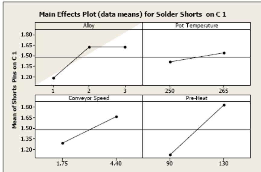
Figure 13 - DOE Main Effect Plots (data means) for Solder Shorts
