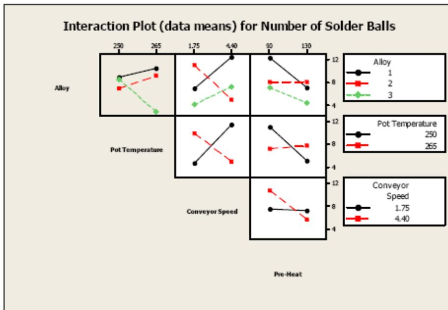
Figure 24 - Interaction Plot from DOE Data (data means) for Solder Balls
