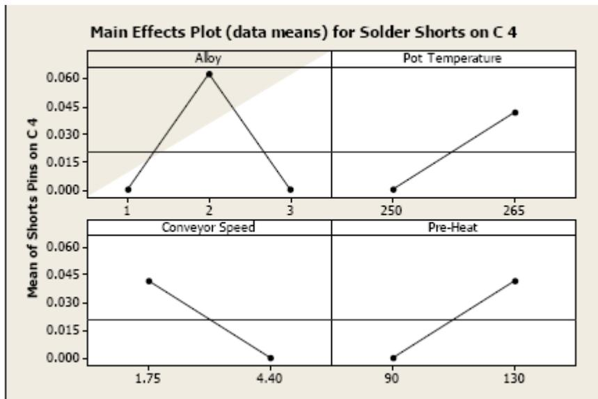
Figure 14 - DOE Main Effect Plots (data means) for Solder Shorts
