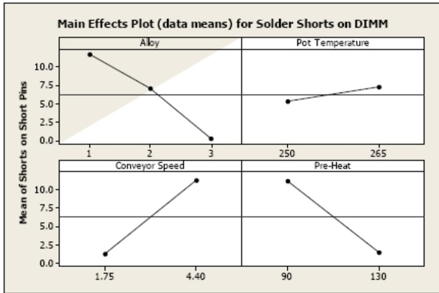
Figure 12 - DOE Main Effect Plots (data means) for Solder Shorts
