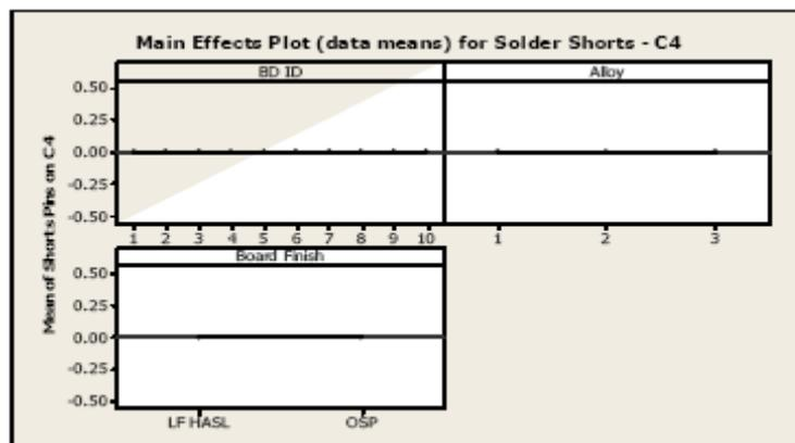
Figure 16 - Confirmation Run Main Effect Plots for Solder Shorts
