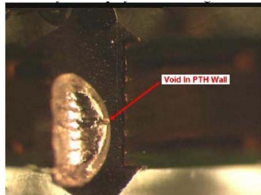
Figure 7 – Exploded View of Wall Imperfection causing the above Void
