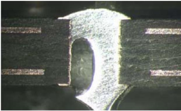
Figure 6 – Micro-Section view of the Subject Void
