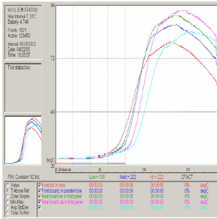
**Figure 4 - Non-Uniform Affect on the Board, with a Wide Temperature Difference across the Panel**
