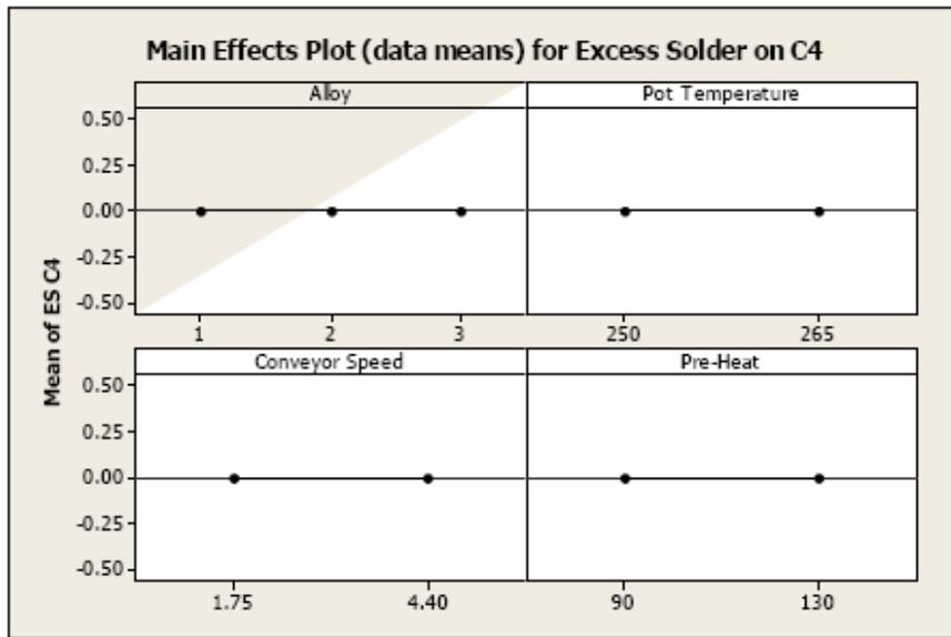
Figure 21 - DOE Main Effect Plots (data means) for Excess Solder (Note: C4 has a thru-board length of 0.175")
