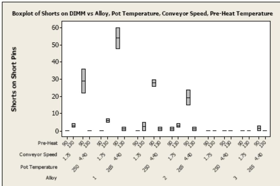
Figure 18 - DOE Box Plot of Solder Shorts on DIMM Connectors (Short Pins)
