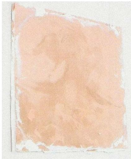
**Figure 1 – Test Plates used to Initially Confirm that the Material could Function as a Capacitor**
