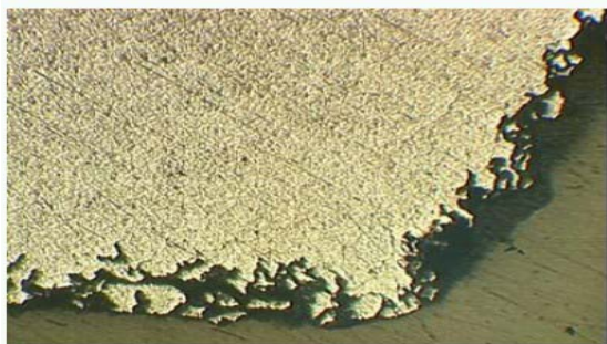
Figure 15 - Tin/lead - Post Cross Section (25X)
