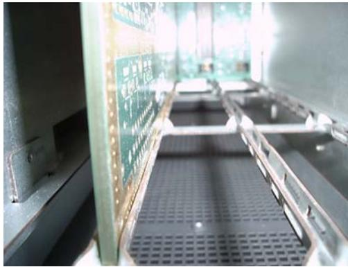
**Figure 8 - Circuit Board in Cabinet Rail**
