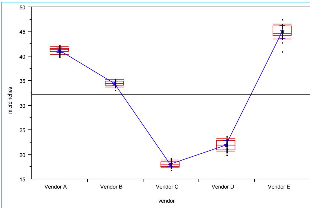
**Figure 3 - Immersion Tin supplied for Wetting Balance Testing**
