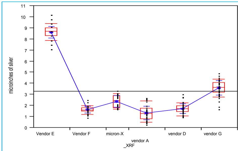
**Figure 5 - Thin Deposit of I Ag XRF Results**
