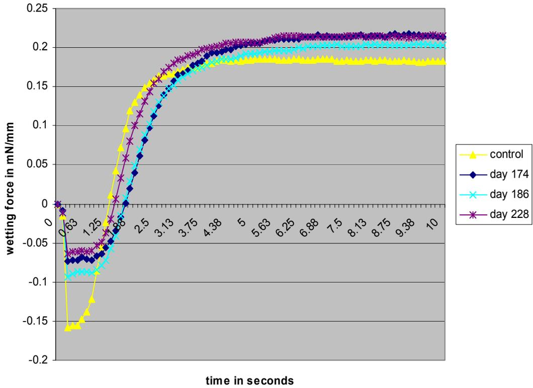
Figure 8 - Supplier A I Sn but Tested at the Lower 215°C Test Temperature
