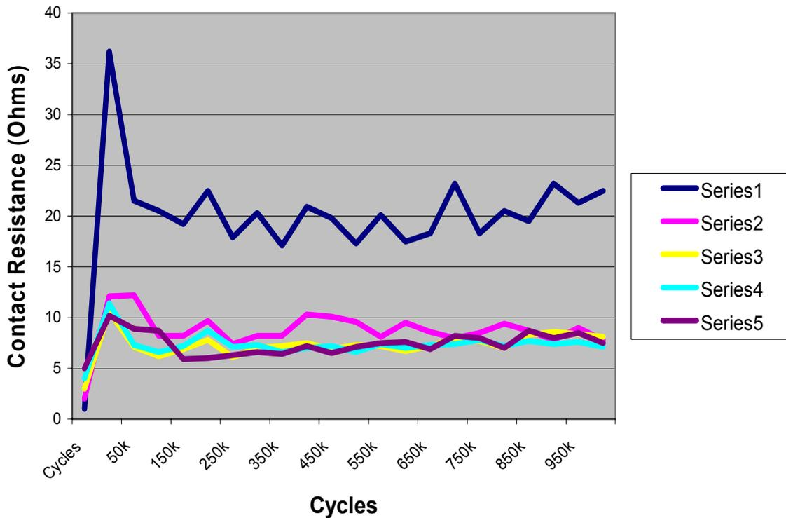
Figure 12 - Contact Resistance Readings for Soft Touch Membrane Switches Tested on Supplier “A” I Ag
