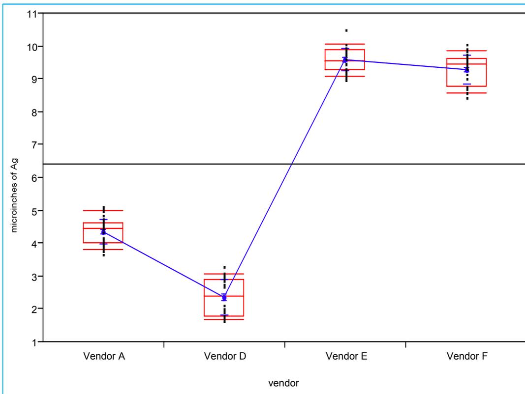
**Figure 4 - Immersion Silver Deposit Supplied For Wetting Balance Testing**
