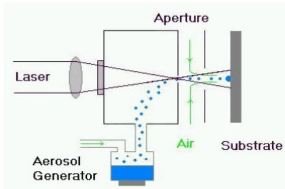
**Figure 2 – Schematic Diagram of the M3D Deposition Head**
