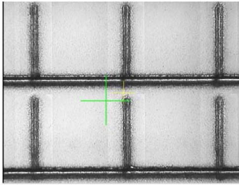
**Figure 7 – Micrograph of Laser Treated Silver Interconnects on PMMA Substrate**
