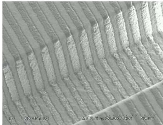
**Figure 5 - Micrograph Showing the Deposition of Silver Ink over a Step Edge and into a Trench**
