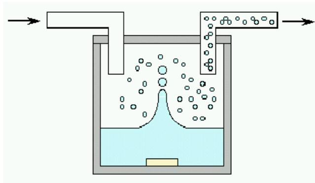
**Figure 1 - Schematic Diagram of the M3D Deposition Process. Liquid Inks and Pastes are First Atomized to Form 1-5  $\mu\text{m}$ -Sized Droplets. The Droplets are Entrained in an Air Stream and Directed Toward a Deposition Head**
