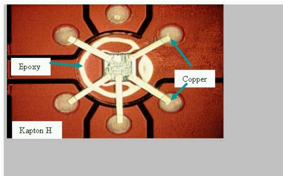
**Figure 8 - Micrograph of Direct Write Silver Interconnects Deposited for Electrically Connecting an IC to a Substrate**
