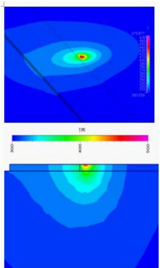
**Figure 6 - Simulation Showing the Localized Heating of a Nanoparticle Ink Film Deposited on PMMA Substrate**
