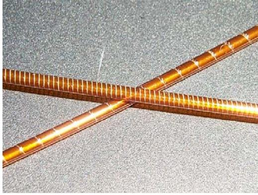
**Figure 9 - Micrograph of Helical Silver Wires Deposited on the Exterior Surface of Polyimide Tubing**
