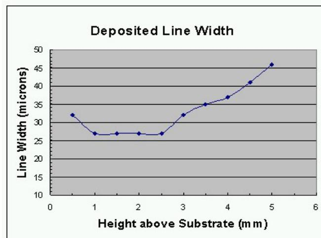
**Figure 4 - Width of Deposited Lines as a Function of Height of the Nozzle above a Substrate**
