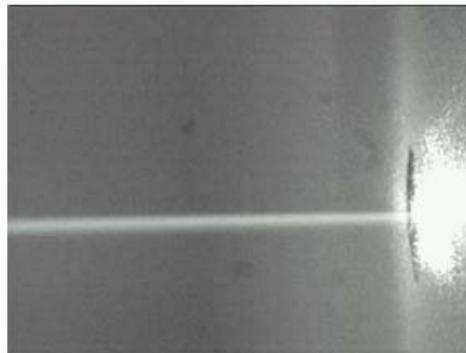
**Figure 3 - Droplet Stream seen Emerging from a 500-micron Diameter Aperture**
