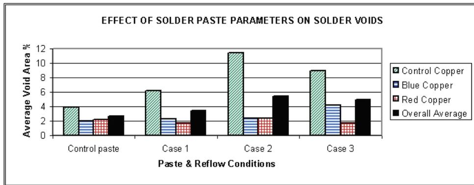
**Figure 14 - Average Void Size Copper Process Versus Paste & Reflow Conditions**
