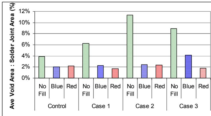
**Figure 8 - Void Size as a Percentage of Solder Joint Cross-sectional Area**
