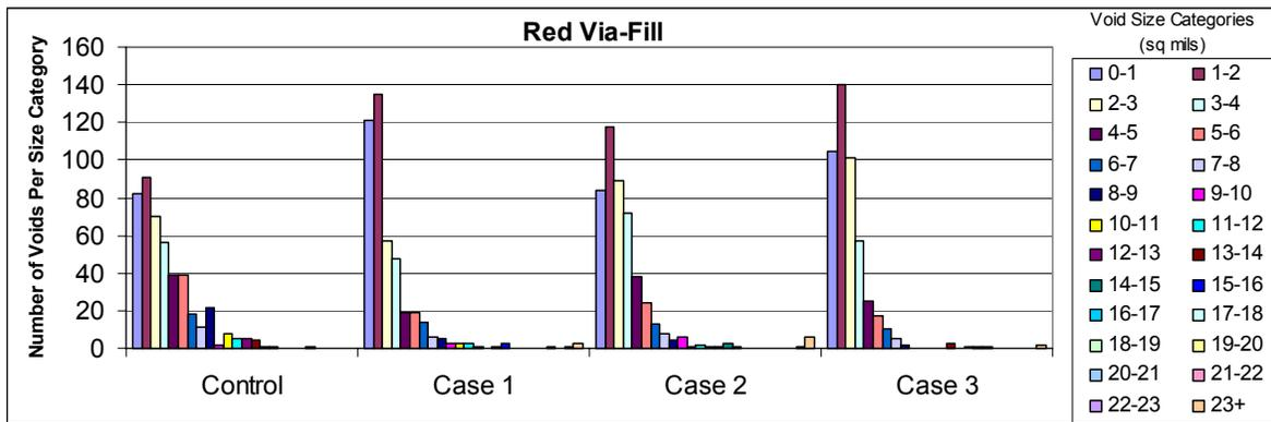
**Figure 13 - Void Frequency Distribution – “Red” (Full) Via-fill**
