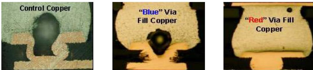
Figure 4 - Three Types of Copper Processes and Variation in Via Fill
