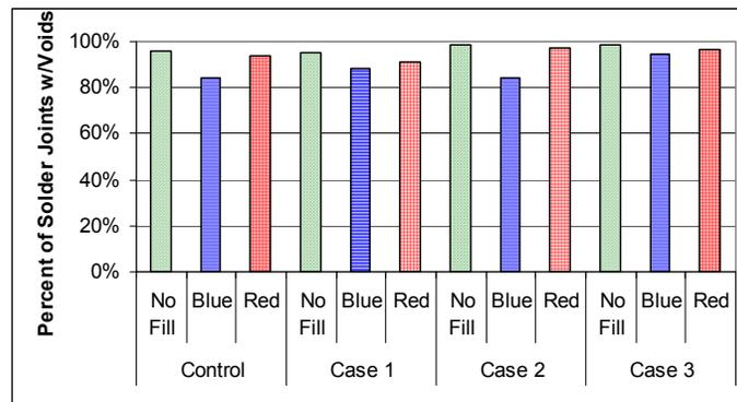
**Figure 9 - Percentage of Solder Joints with Voids (X-ray data)**
