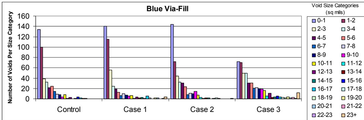
**Figure 12 - Void Frequency Distribution – “Blue” (Partial) Via-fill**
