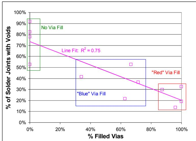
**Figure 6 - Cross-section Data: Comparing Void Occurrence with Via-Fill Success**
