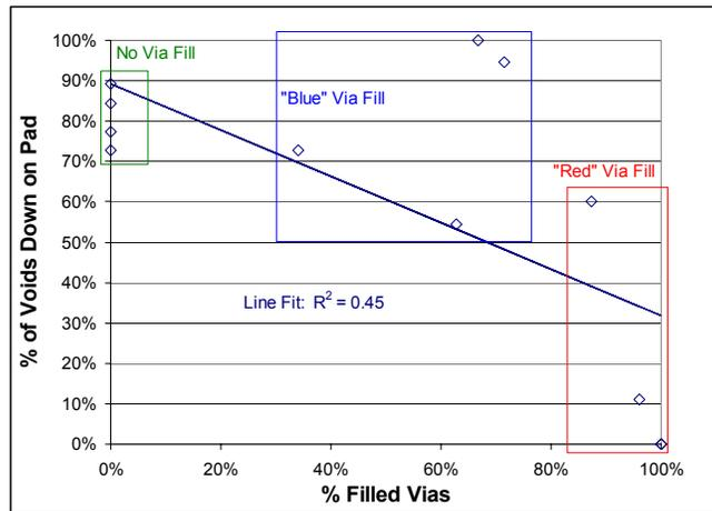
**Figure 7 - Cross-section Data: Comparing Void Height with Via Fill Success**
