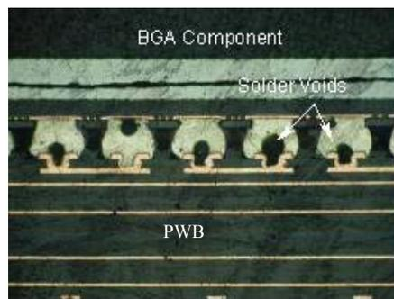
**Figure 1 - Solder Voids From Via-in-pad Designs**
