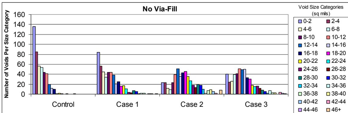
Figure 11 - Void Frequency Distribution – No Via-fill- Control Copper
