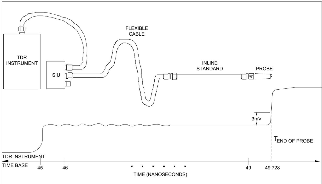
Figure 2 – Multiple: Find End of Probe
