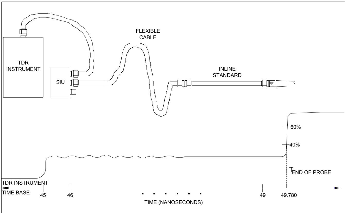
**Figure 8 - TM-650: Find end of Probe**
