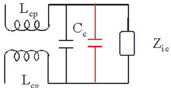
Figure 2 – Decoupling (bypass) Capacitor
