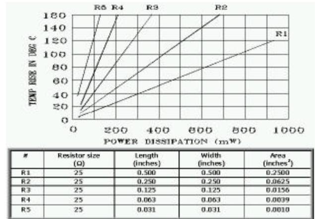
Figure 10 – Effect of Resistor Size of Heat Generation
