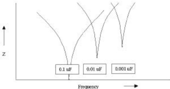
**Figure 3 – Low Resonant Frequency**
