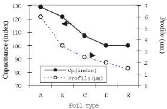
**Figure 2 - Copper Foil Type and Capacitance**
