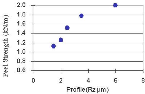
**Figure 1 – Relation between Copper Profile and Peel Strength on Standard Epoxy Resin System**
