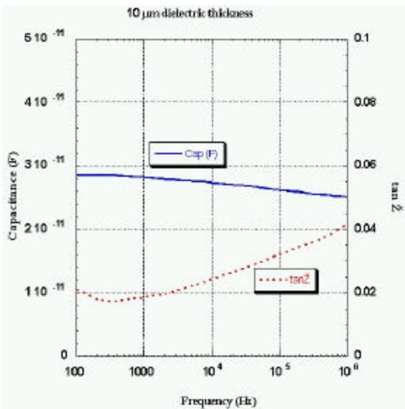
**Figure 10 – Capacitance of 10 μm Core vs. Frequency**
