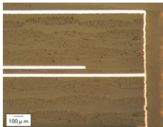
**Figure 5 - Cross-Section of Board Using 50µm Capacitive Core as a Reference**
