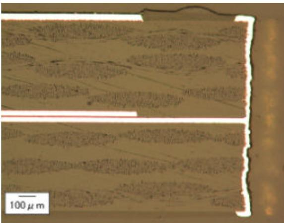
**Figure 7 - Cross-Section of Board Using 10 µm Capacitance Layer**
