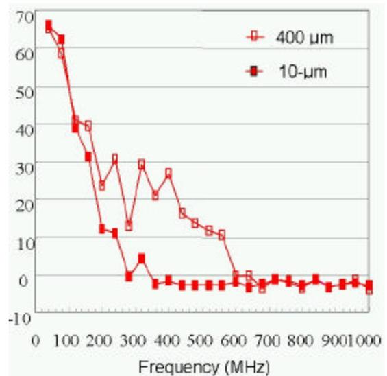
**Figure 9 – Comparison of Noise Current with Standard Laminate Core and 10 µm Core<sup>4)</sup>**
