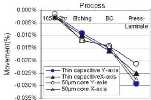
**Figure 4 – Dimensional Stability During the Process**
