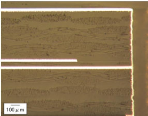
**Figure 6 - Cross-Section of Board Using 25µm Capacitive Layer**
