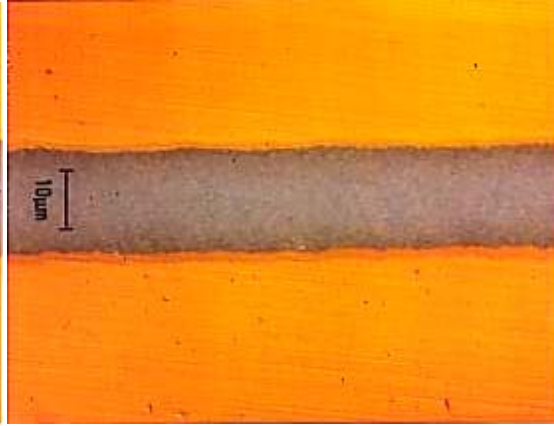
Foil D R_z=2.0\ \mu\text{m}
