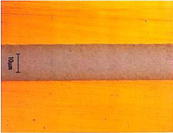
Foil E R_z=1.5\ \mu\text{m}
