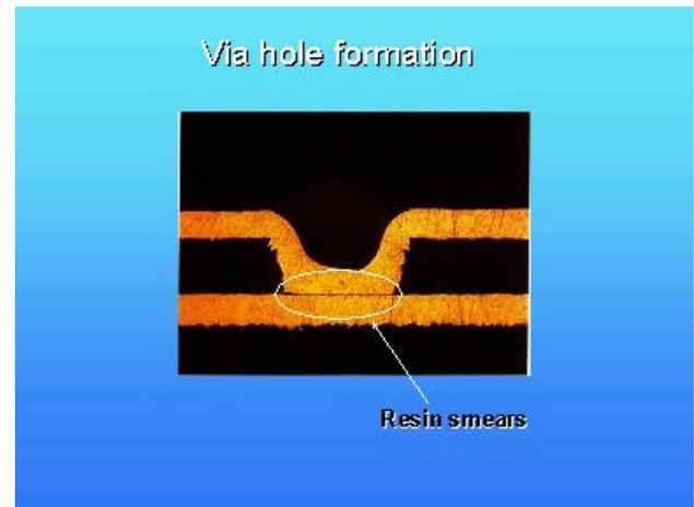
**Figure 1 - Microvia after Plating that has Residual Smear from the Formation Process**
