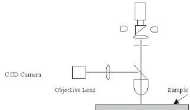
**Figure 5 - Basic Schematic of Equipment Set Up**
