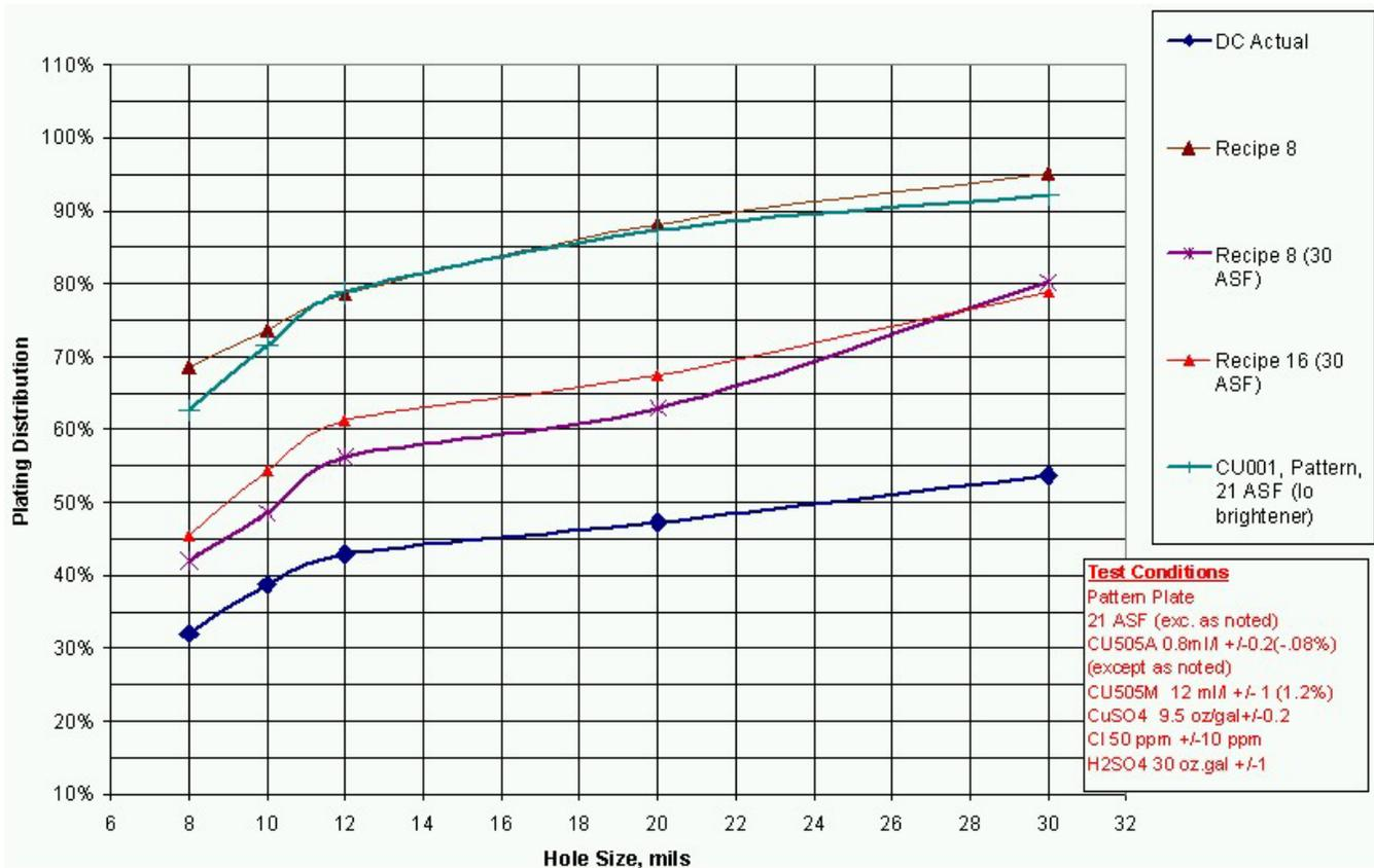
Figure 4 - Plating Distribution vs. Hole Size in ~0.125” Panel
