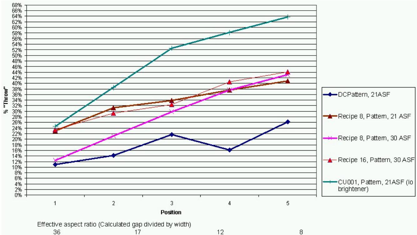
Figure 3 – Test Cell Results Percent “Throw” vs. Aspect Ratio
