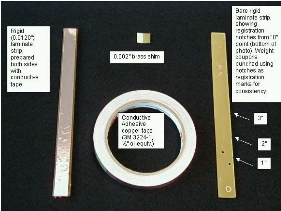
Figure 1 – Equipment for Fixing Distances
