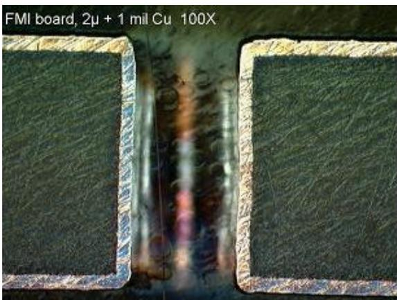
**Figure 13 – Metallized Via with Shadow® followed by Electrolytic Copper Plating**
