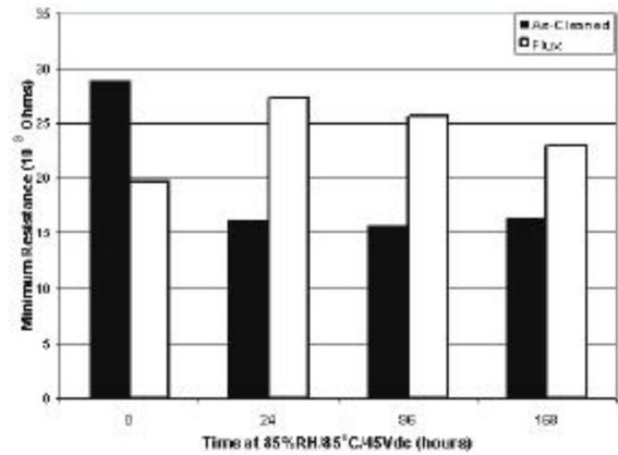
Figure 17 - Minimum SIR Test Results
