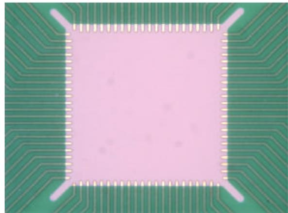
Figure 18 - Flip Chip Assembly Site
