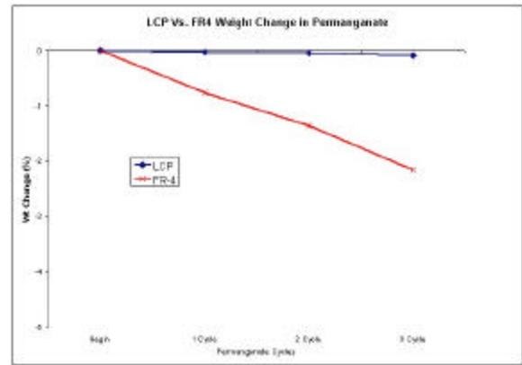
**Figure 10 – Weight Loss through Permanganate Exposure**
