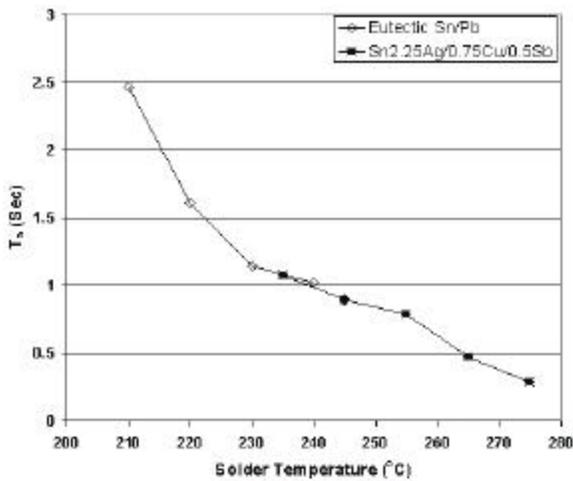
Figure 15 -  $T_a$  as a Function of Temperature for the Two Solder Alloys
