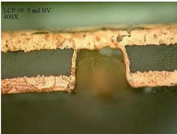
**Figure 12 – Metallized Via with Electroless followed by Electrolytic Copper Plating**
