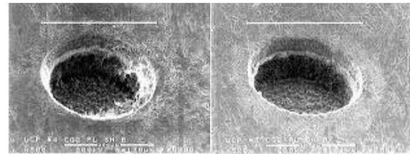
**Figure 11 – LCP as Drilled (left) – After Plasma Desmear (right)**
