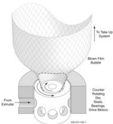
**Figure 3 - Biaxial Orientation is Achieved Using the Counter Rotating Circular Die**
