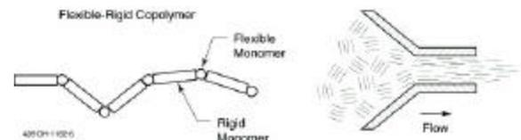
**Figure 1 - Liquid Crystal Polymers have Rigid Segments, which tend to Align in Shear Flow**
