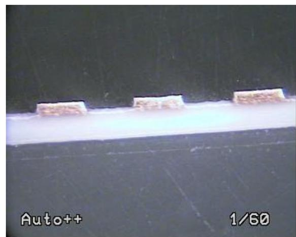
**Figure 4 – Cross-Section LCP Circuit Traces (Courtesy of Mound Flextek)**
