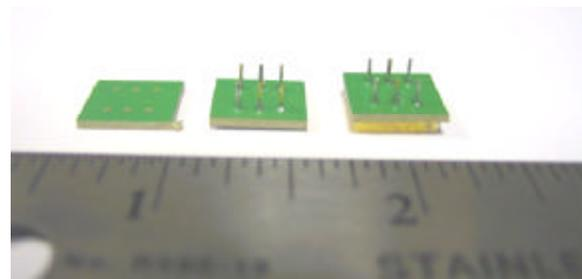
**Figure 23 - LCP MEMS Package.**
