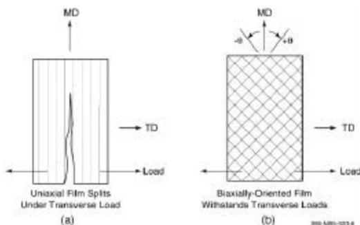
**Figure 2 – Comparison of Uniaxially and Biaxially Oriented LCP Film**
