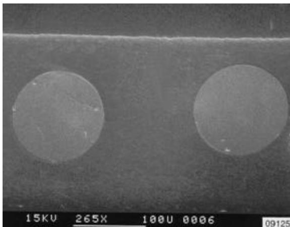
**Figure 27. Scanning Electron Micrograph of Optical Fibers Through LCP Package Wall**
