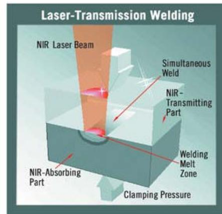
Figure 24 - Laser Welding of Thermoplastics<sup>9</sup>
