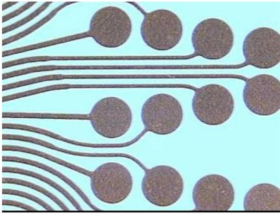
**Figure 5 – LCP Circuitry – Traces and Pads**
