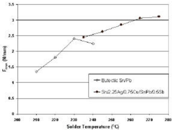
Figure 16 -  $F_{max}$  as a Function of Temperature for the Two Solder Alloys
