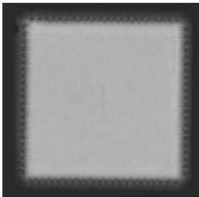
**Figure 20 - Typical C-SAM Image After Underfill and Cure**
