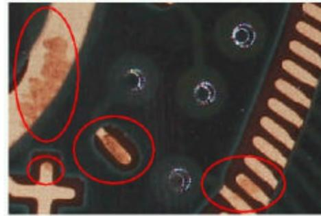
Figure 3 - Defects on PBGA Gold Surface
