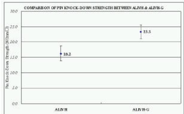
**Figure 28 - Pin Knock-Down Strength Test**
