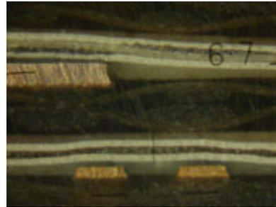
**Figure 6 - PTFE/Fiberglass/BT-Epoxy Prepreg Filling 1& 2 oz Circuitry [35 wt% BT Resin, 4°F(2°C)/min Heat Rise].**
