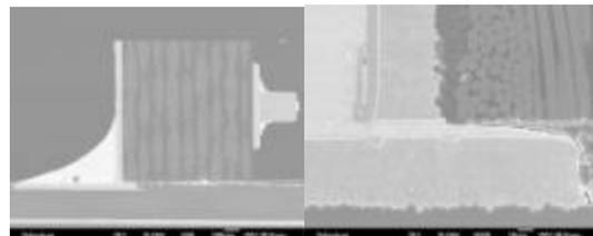
**Figure 9 - SEM Image of SAC Soldered LED – Good Solder Joint (5mils Stencil)**
