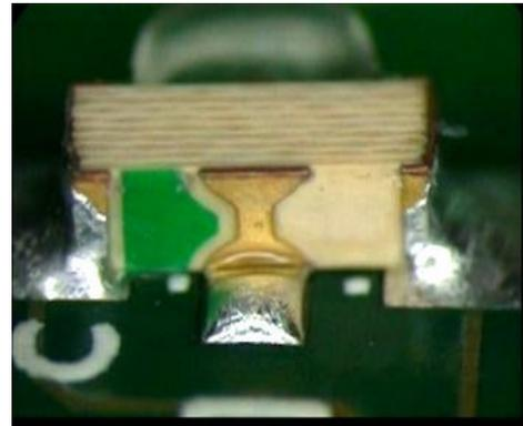
**Figure 4 - Image of Non-Wetting SAC Soldered LED**
