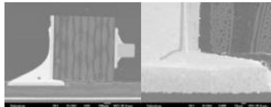
**Figure 10 - SEM Image of SAC Soldered LED – Good Solder Joint (6mils Stencil)**
