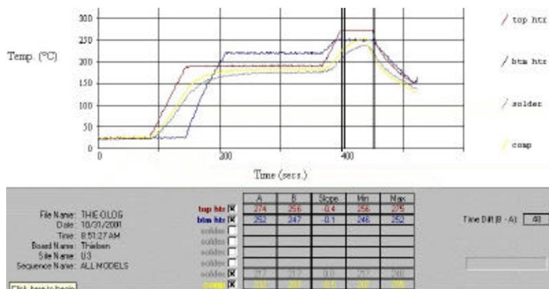
Figure 2a- SAC Rework Profile – Solder Joint
