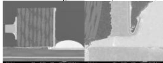
**Figure 8 - SEM Image of SAC Soldered LED – Non-Wetting Solder Joint (6mils Stencil)**
