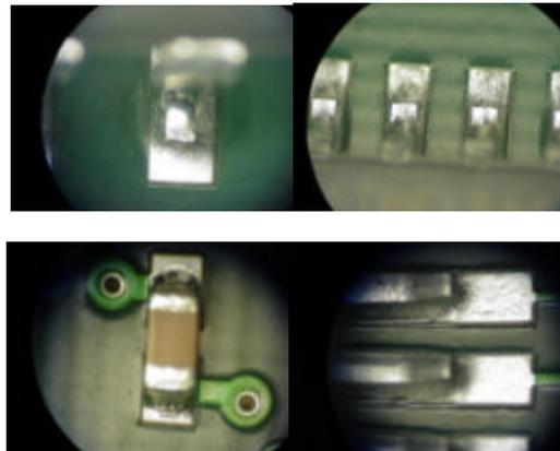
**Figure 12- Images of good SAC Solder Joints Observed**
