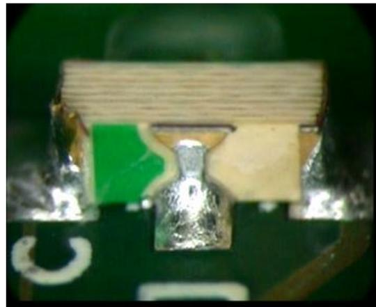
**Figure 6 - Image of Good Wetting for SAC Soldered LED**
