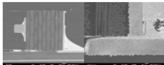
**Figure 11 - SEM Image of SnPb Soldered LED – Good Solder Joint (5mils Stencil)**
