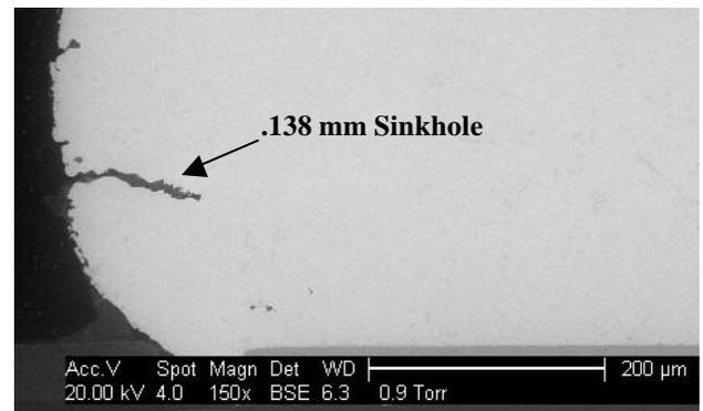
**Figure 25 – Sinkhole Void Sn/Ag/Cu/Sb Solder Joint after 12500 Cycles (30 min. cycles)**
