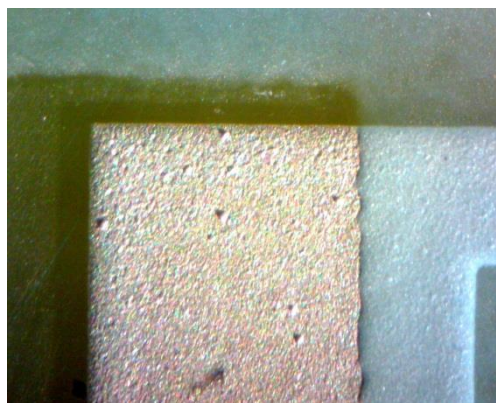
Figure 3. Pad partially covered with UV dielectric
