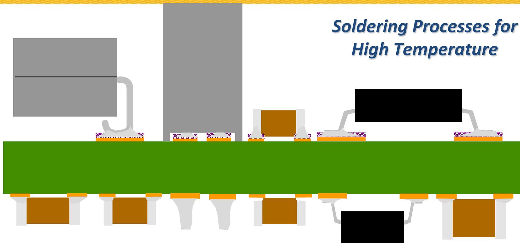
Assembly process is limited by the PCB and component temperature range
