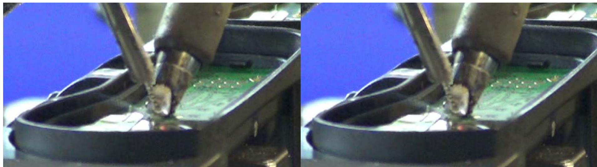
Example of customers soldering operation on surface mount module with through hole terminations. The second video is in slow motion to show the process steps more clearly
