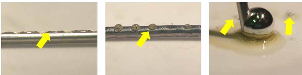
Figure 10: Images above left & centre show the point that flux escapes from the wire during heating. On the right solder balls formed on a white ceramic tile when the wire was not prepared
