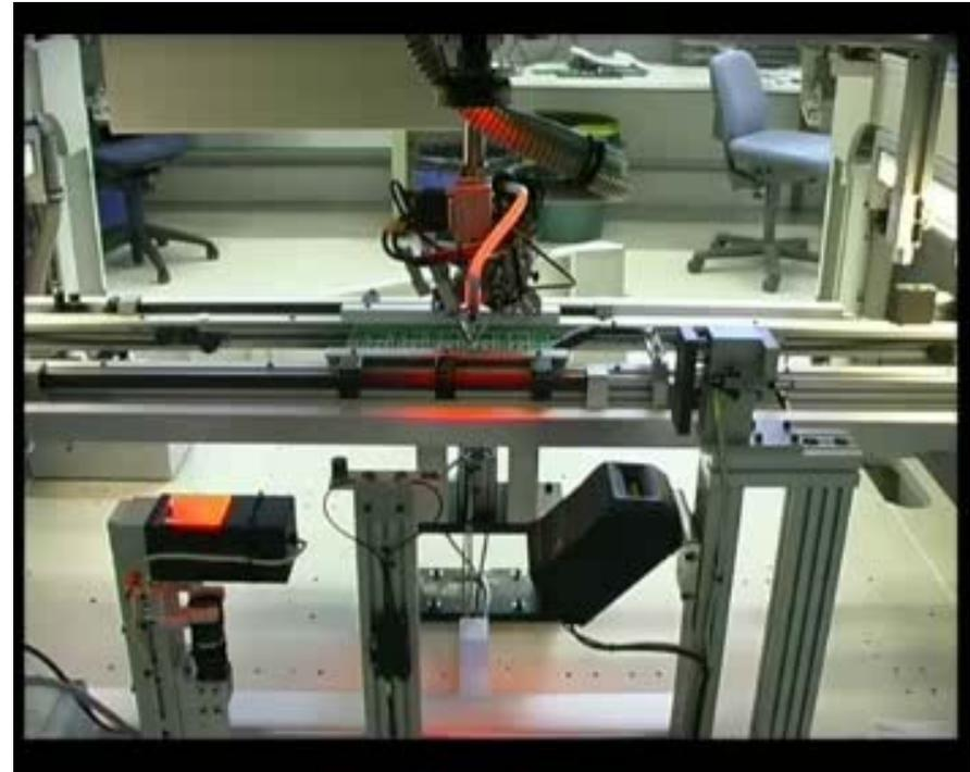
Robotic iron soldering
