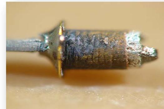
Pull out of copper barrel
