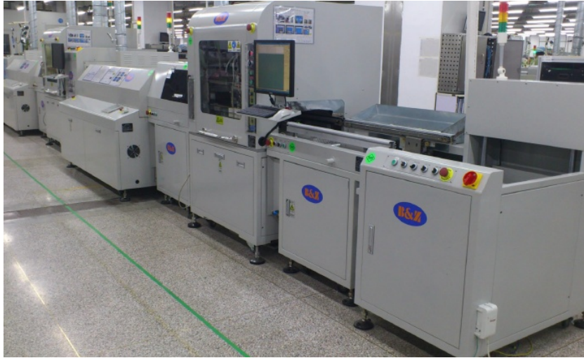
Figure11: Corrosion-resistant conformal coating equipment
