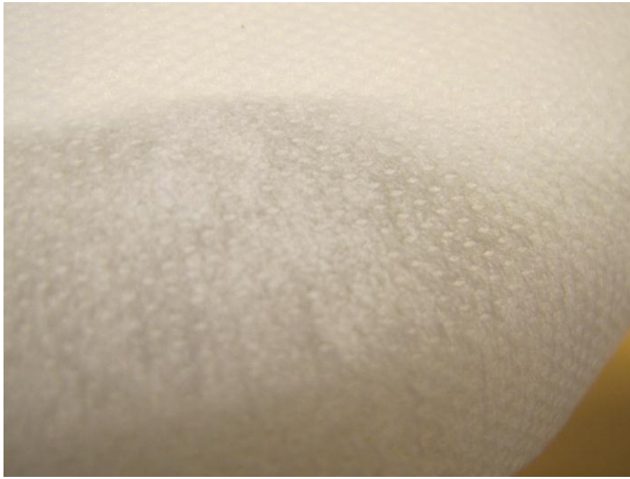
Figure 7 – Photo of cleaning paper B. Wave formed surface because of regular imprints.
