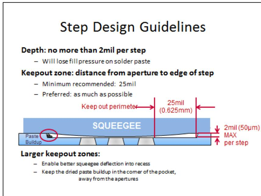
**Figure 3. Alternate Stencil Step Down Design Guidelines<sup>4</sup>**
