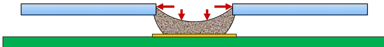
At separation, the forces holding the deposit to the pad must overcome the forces holding the deposit to the stencil walls
