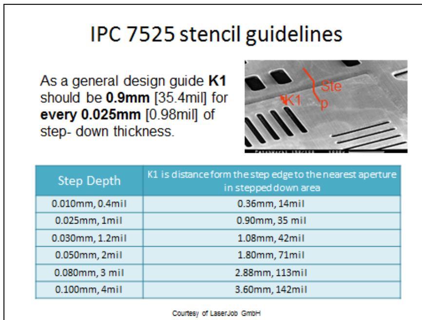
**Figure 2. IPC-7525 Stencil Step Down Design Guidelines<sup>2</sup>**
