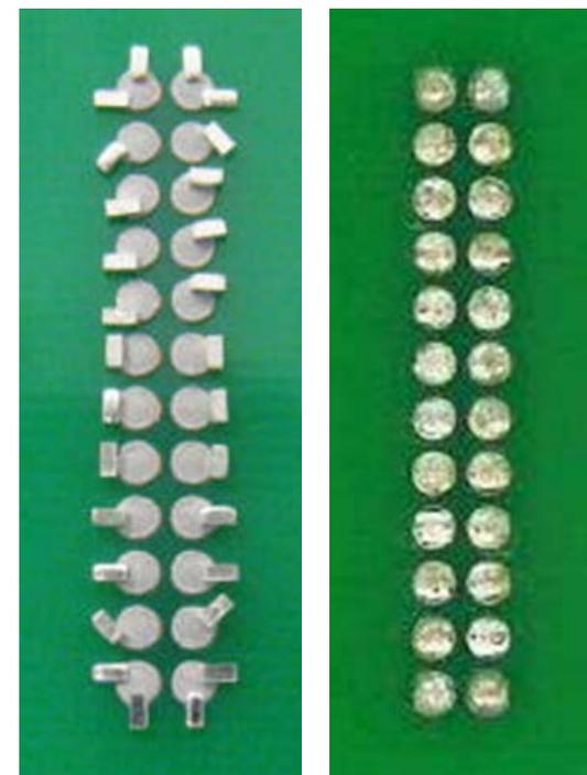
Solder preforms placed in solder paste add volume to PTH and other large solder joints
