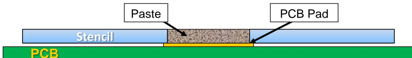
After the aperture is filled, the solder paste sets up and sticks to both the stencil walls and the pads.
