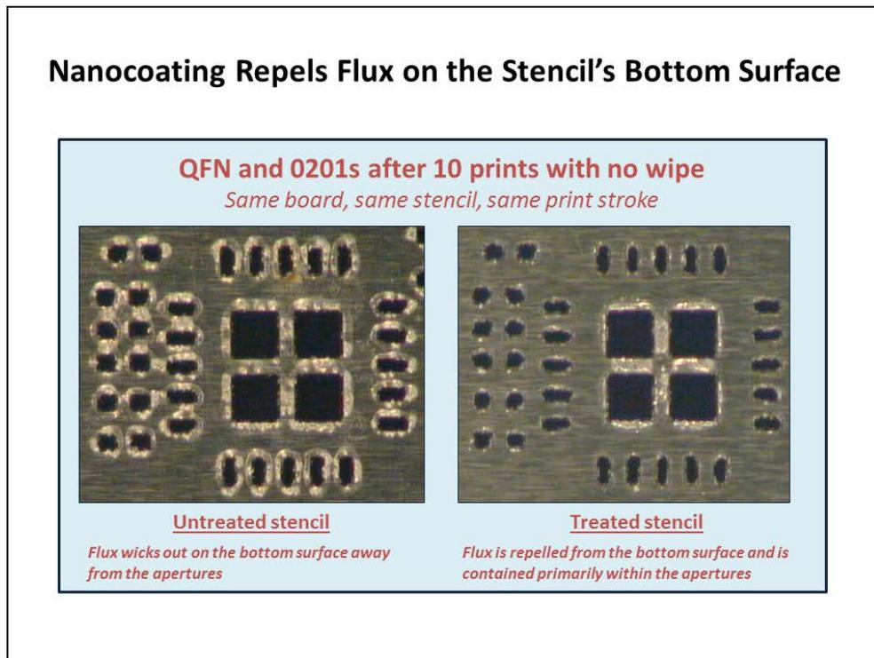
**Figure 7. Flux spread on stencil bottom after 10 prints**
