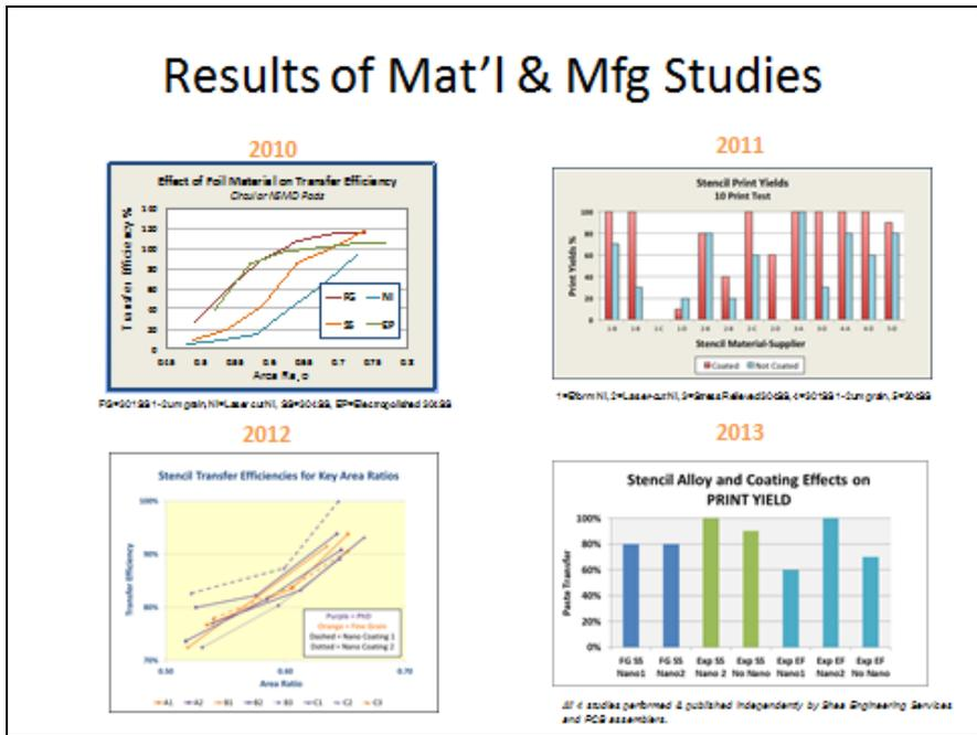
Figure 5. Results of print tests comparing foil materials
