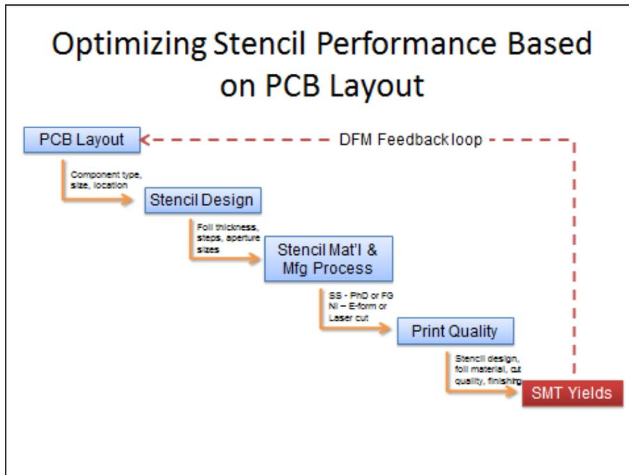
Figure 1. Overview of stencil optimization process<sup>1</sup>
