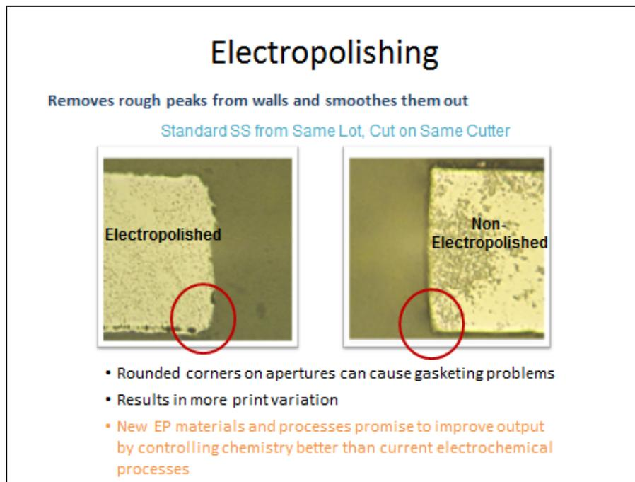
**Figure 6. Cross sections of electropolished stainless steel apertures**
