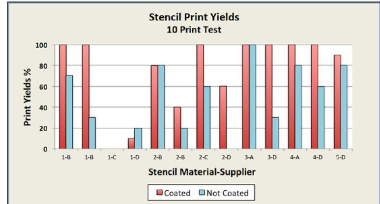
1=Eform Ni, 2=Laser-cut Ni, 3=Stress Relieved 304SS, 4=301SS 1-2um grain, 5=304SS
