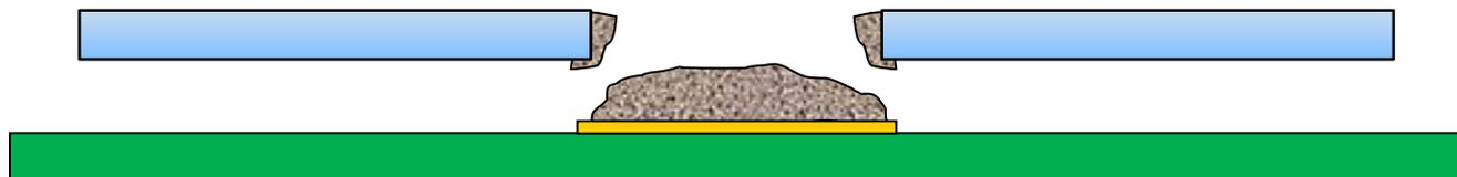
Depending on area ratio, a portion of the paste will release to the PWB, while some will stay in the aperture. Some paste may also stick to the bottom of the stencil due to stringing, bad gasketing or pump out
