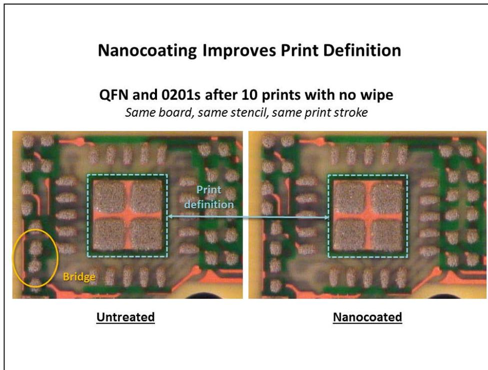
**Figure 8. Print definition with and without nanocoating**
