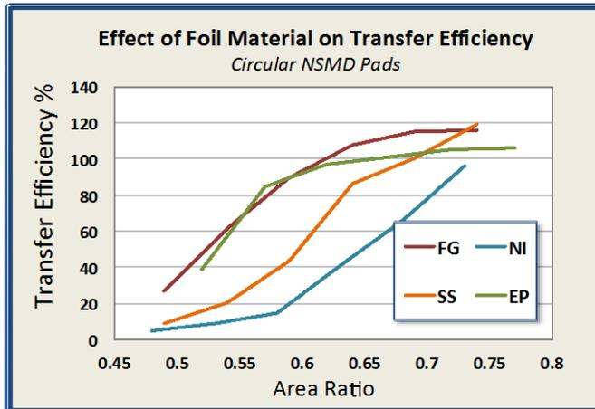
FG=301SS 1-2um grain, NI=Laser cut Ni, SS=304SS, EP=Electropolished 304SS
