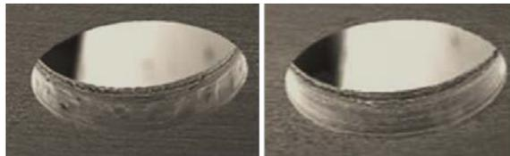
**Figure 3. Flexible PI PTH. Electroless copper (left) and electroless copper with stress reducing additives (right)**
