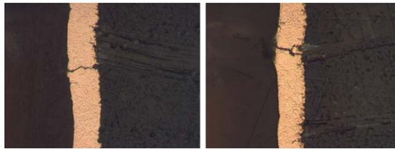
**Figure 6. Examples of IST sense circuit failures identified by cross section evaluation as copper plating cracks.**
