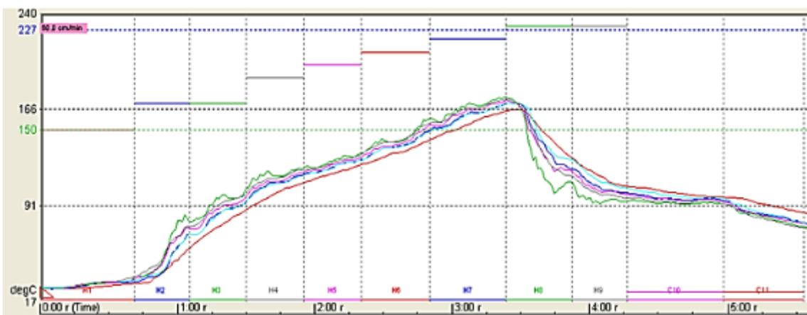
Low-temperature reflow profile used for solder paste material F
