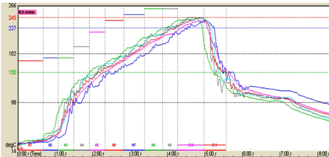
High-temperature reflow profile used for solder paste materials A-E
