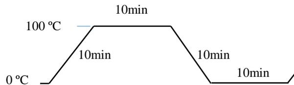
Figure 6. Thermal Cycle Temperature Profile – 0 °C to 100 °C
