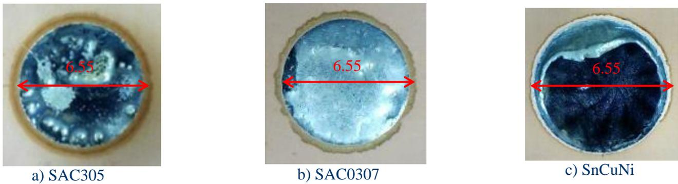
**Figure 2 – Wetting Test Results of Various Lead-Free Alloy Solder Pastes. The images of Wetting Test for a SAC305, SAC0307 and SnCuNi alloy solder paste were shown. These three solder pastes had on average a similar spreading diameter.**
