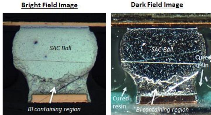
Figure 14 – Bright Field and Dark Field Optical Micrographs for a BGA LTRR solder joint
