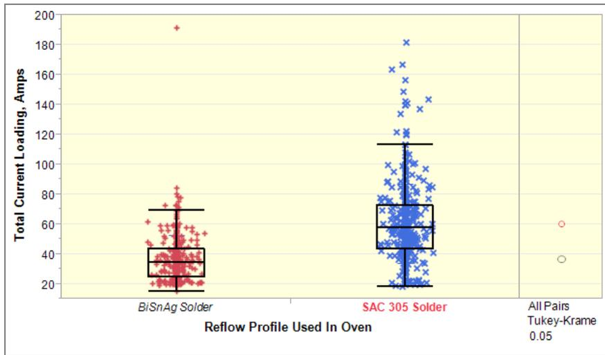
**Figure 17 – Comparison of Current Loading for a Reflow Oven when running a Low Temperature BSA soldering vs a standard SAC soldering reflow profiles**
