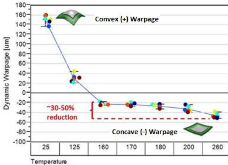
**Figure 3 – Dynamic Warpage plot with temperature for a FCBGA package. The amount of dynamic warpage reduction if soldering in the 160-180C peak reflow temperature range is indicated**
