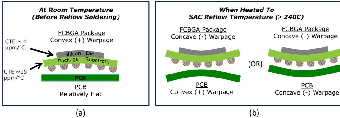
**Figure 1-Typical warpage shapes of FCBGA packages (a) at room temperature and (b) at SAC solder paste reflow temperatures**
