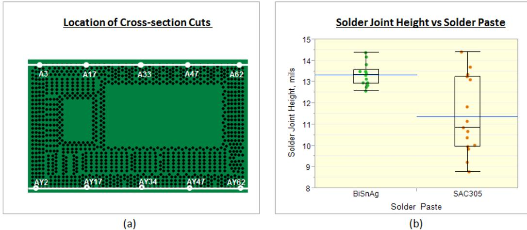
**Figure 10 - (a) Location of the two cross-section cuts made within the ball array of the BGA package TV1; (b) Solder Joint Heights for the BGA package TVs vs the solder paste type used to assemble them.**
