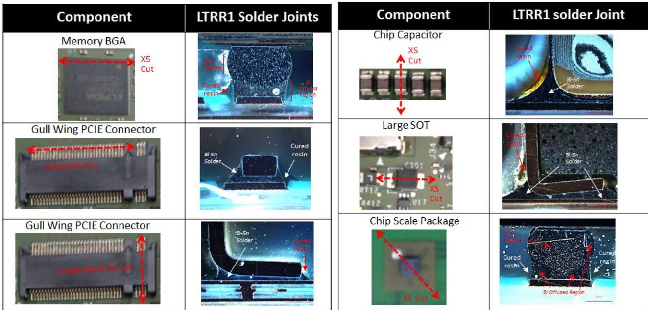
Figure 15 –Dark Field Images of Optical Micrographs for a BGA solder joint formed using LTRR solder paste.
