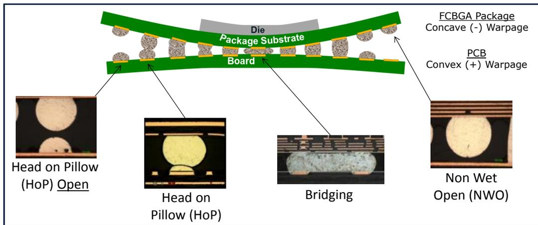
**Figure 2 - Description of defects that can be caused by dynamic warpage of FCBGA components and/or PCBs during the reflow soldering process**
