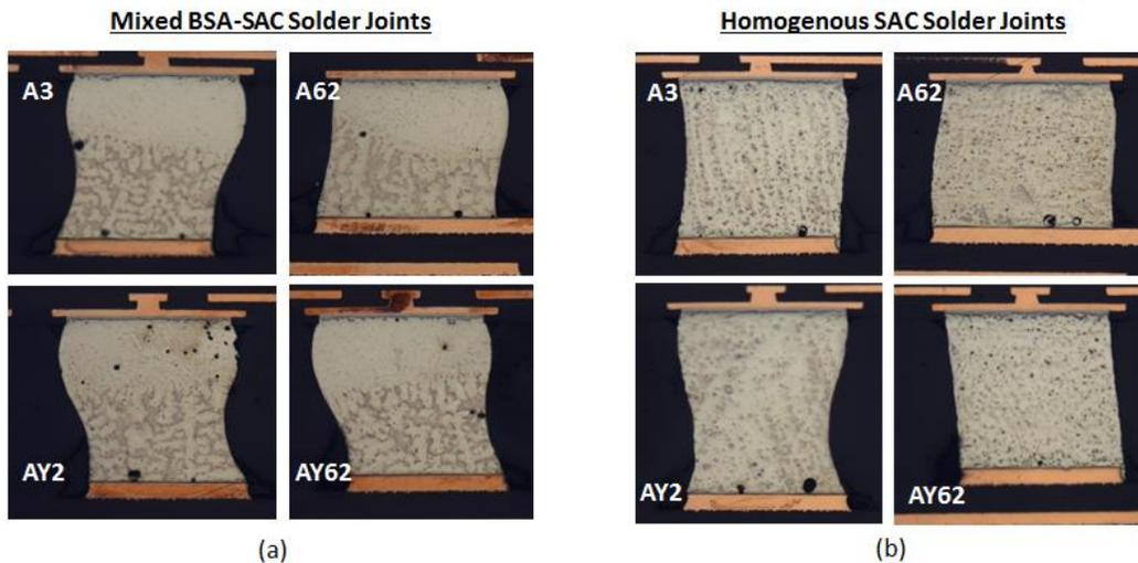
**Figure 11 – Optical Microscopy Images of Solder Joint Cross-sections at the Four Corners of the BGA TV1. (a) BSA solder paste and reflow profile was used to form these solder joints; (b) SAC solder paste and reflow profile was used to form these solder joints**
