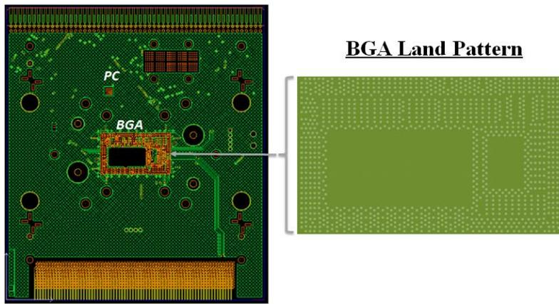
Figure 6 - The printed circuit board test vehicle used and a magnified view of the BGA land pattern used for evaluation of the printing capabilities of the solder pastes.
