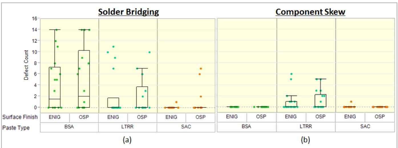
**Figure 13 - Comparison of Defects at 0.100mm Component Spacing due to (a) Solder Bridging and (b) Component Skew**
