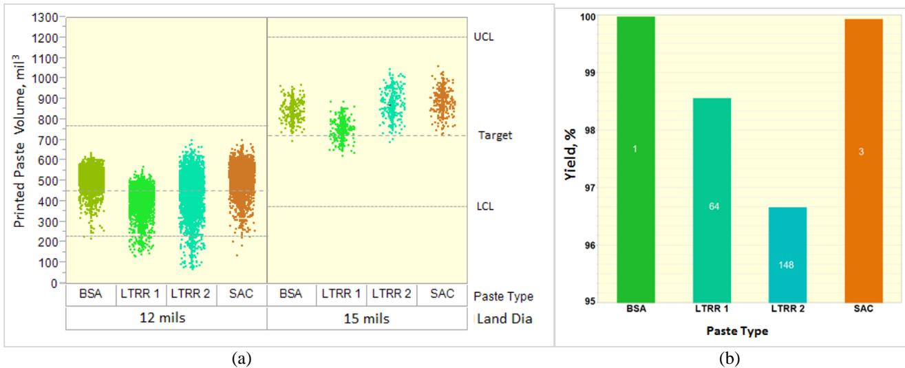
Figure 7 - (a) Printed Paste Volume in cubic mils for each solder paste evaluated on 12 and 15 mils diameter lands; (b) % Yield at the land level, for each solder paste evaluated for the 12 mils diameter lands.
