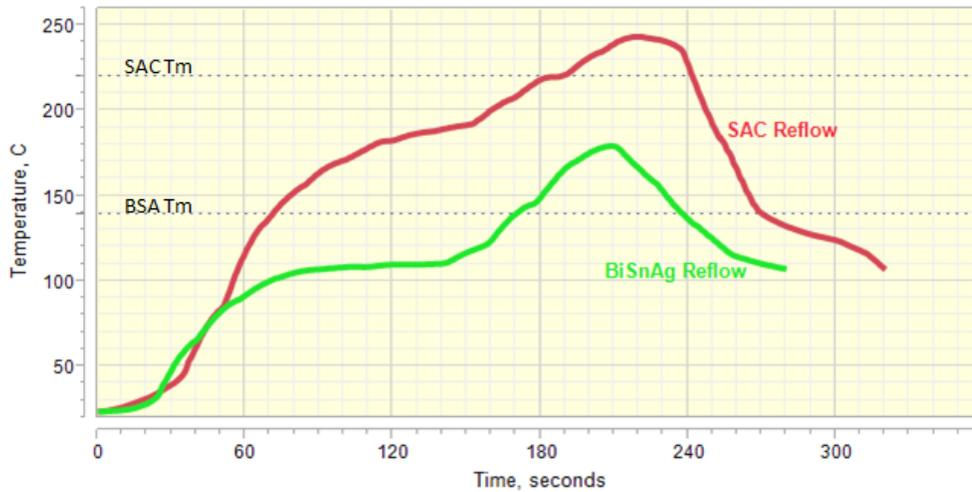
**Figure 16 - The Two Reflow Profiles used for the Power Use Savings Study**
