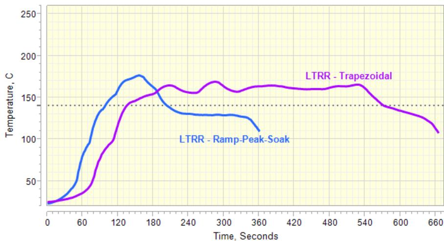
Figure 18 – Comparison of the Ramp-Peak-Soak Reflow Profile to the Trapezoidal profile for LTRR solder pastes
