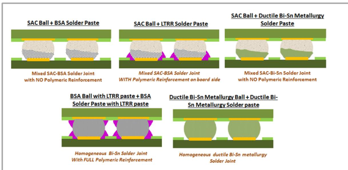
Figure 19 – Various BGA Solder Joint Configurations, using low temperature Bi-Sn solder pastes, which will be evaluated for assembly feasibility and reliability as part of future work
