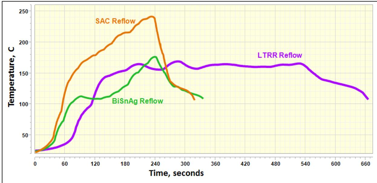
**Figure 5 – Comparison of Reflow Soldering Profiles for the Three Types of Solder Pastes (SAC, BSA, LTRR) evaluated.**
