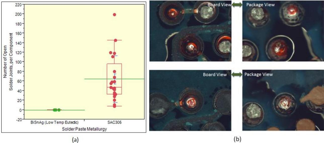
**Figure 9 - (a) Number of Open Solder Joints per component for eutectic BiSnAg and SAC305 solder paste metallurgies; (b) Optical Micrographs of the surfaces of boards and components, post Dye and Pry, for two failed components.**
