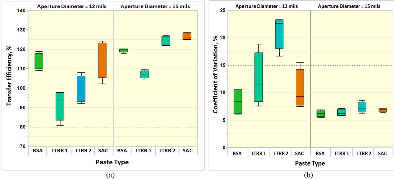
**Figure 8 - (a) Mean of Transfer Efficiency for each solder paste evaluated on 12 and 15 mils diameter lands; (b) Mean of the Coefficient of Variation for each solder paste evaluated for the 12 mils diameter lands.**
