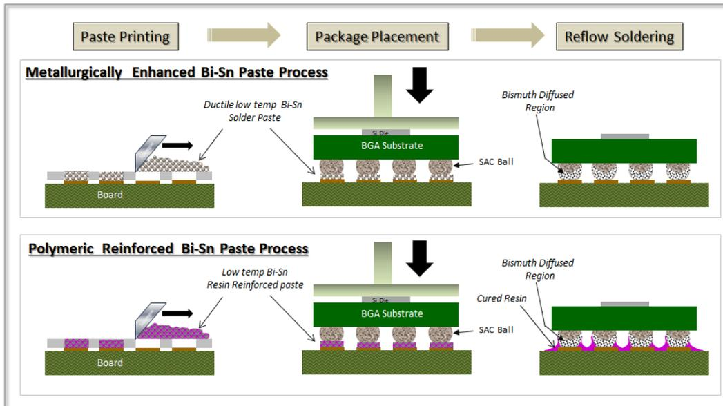
**Figure 4 – Comparison of Assembly Process Steps for Metallurgical and Polymeric Enhancement of Low Temperature Bi-Sn Solder Joints for BGA components**
