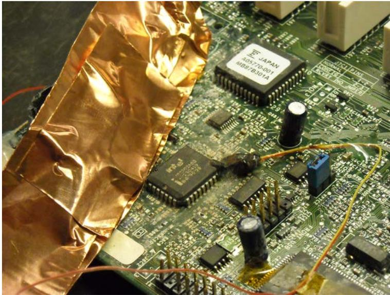
*Figure 7-Copper shielding tape*
