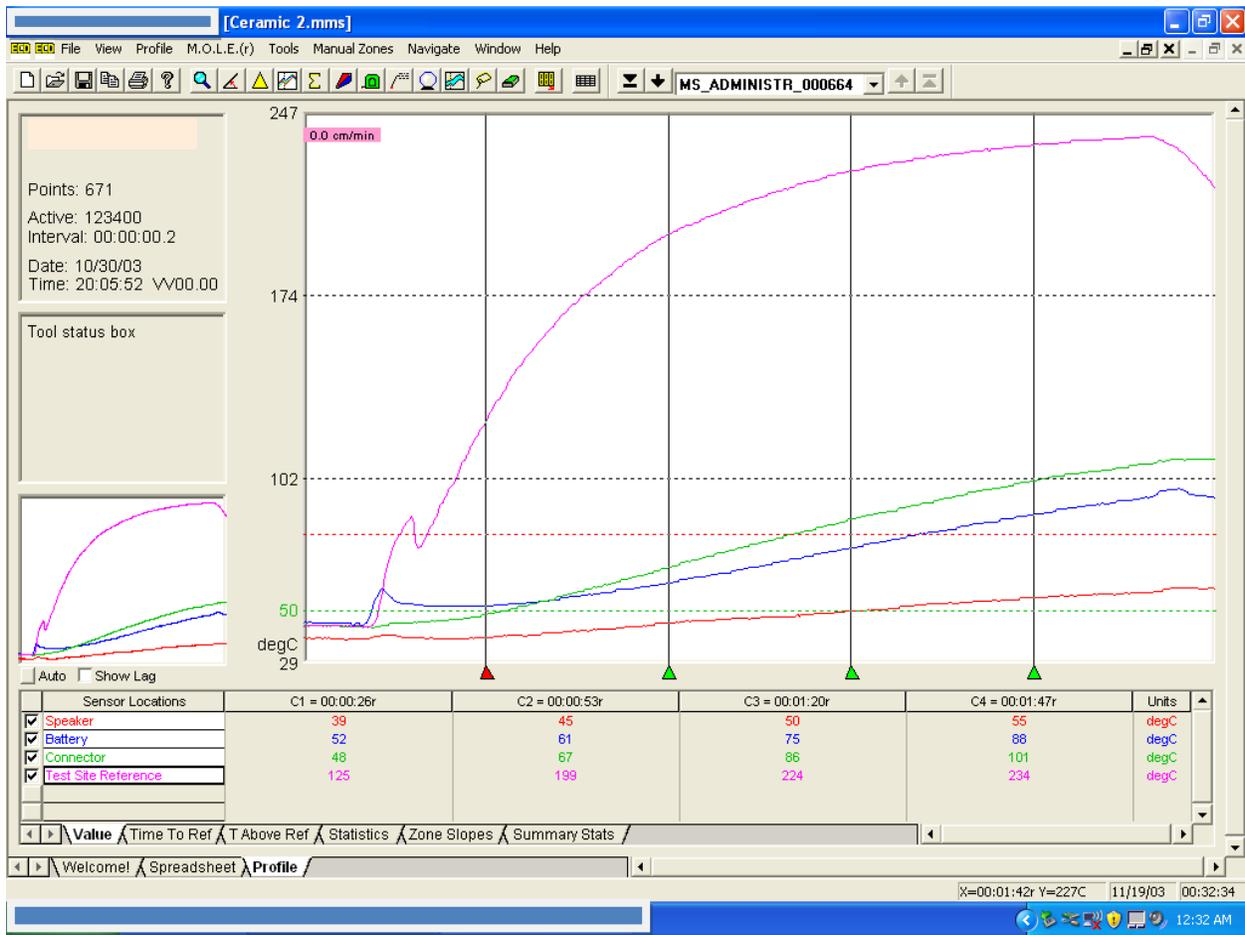
**Figure 3-Sample output reflow profile**
