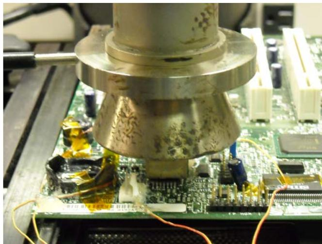
*Figure 6- Hot air nozzle placed over reference location*
