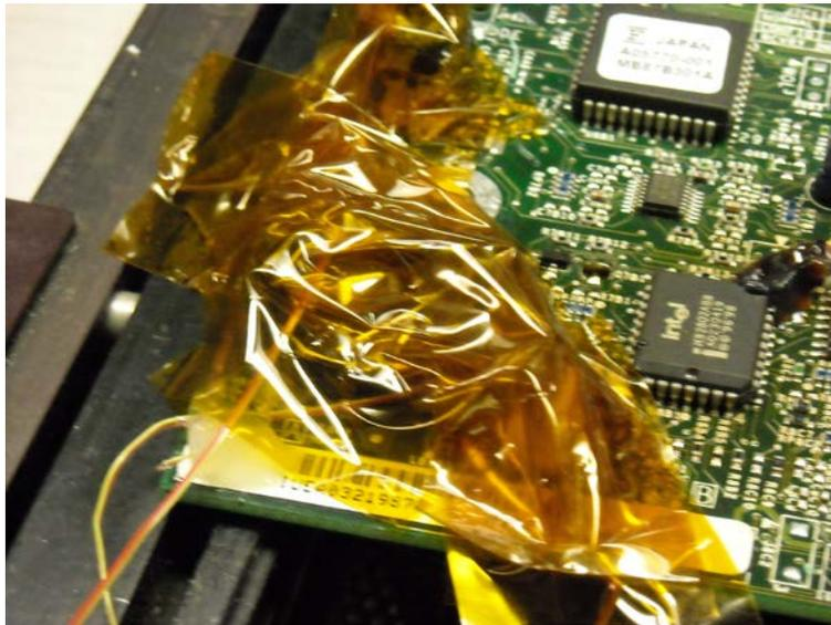
*Figure 9-Kapton tape used as a shielding material*
