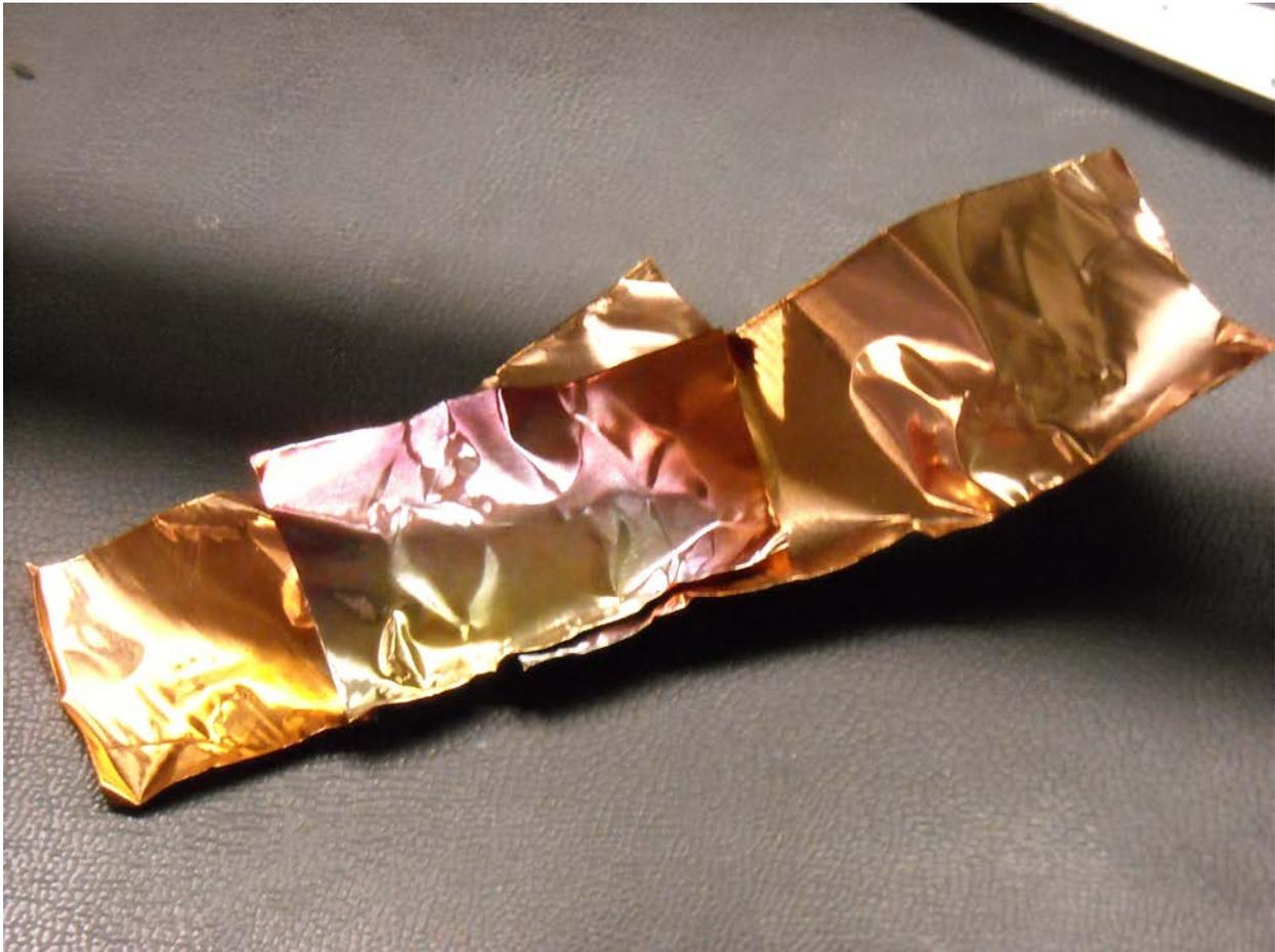
*Figure 8-After repeated heat cycles copper tape discolors*
