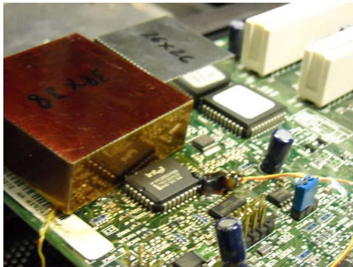
*Figure 10-Stainless steel shields used in study*
