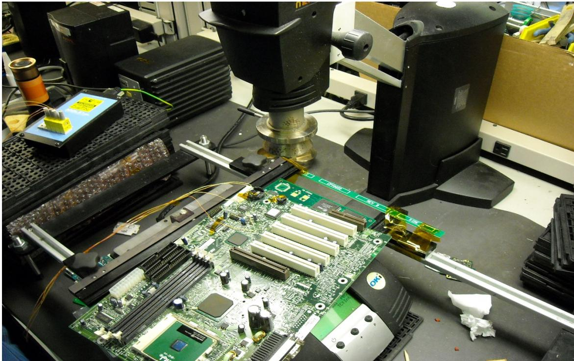
*Figure 1-Board used for testing fitted to board holder of hot air rework system*
