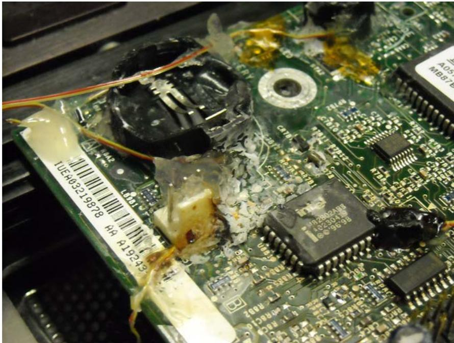
*Figure 12-The gel easily conforms to openings and gaps. It discolors after being heated.*
