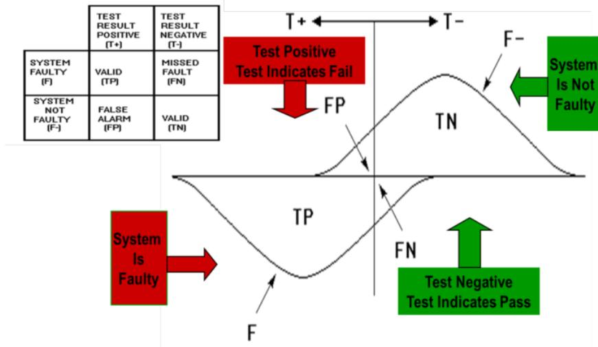
Figure 3 - Graphical representation of possible test outcomes [1]
