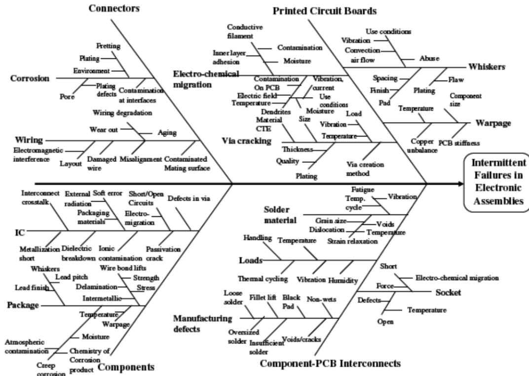
Figure 2 – Cause-and-effect diagram of intermittent failures in electronic assemblies [2]
