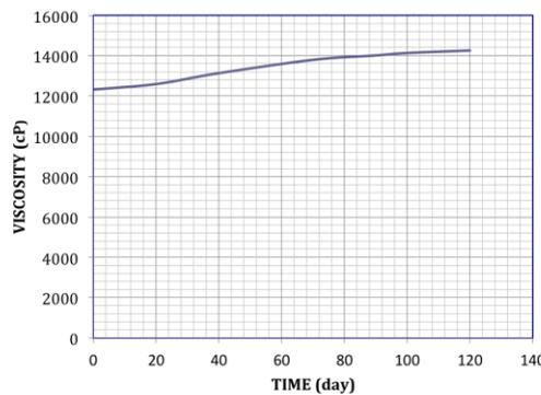
Fig.6 Viscosity of SJEA Changing With Storage Time
