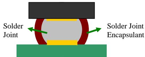
Fig.2 Schematic of Cured SJEA Encapsulated Solder Joint
