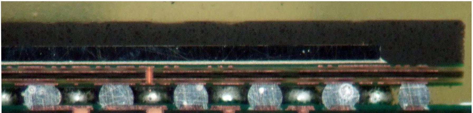
Diagonal cross section of soldered part. Note outer balls are taller than center balls.
