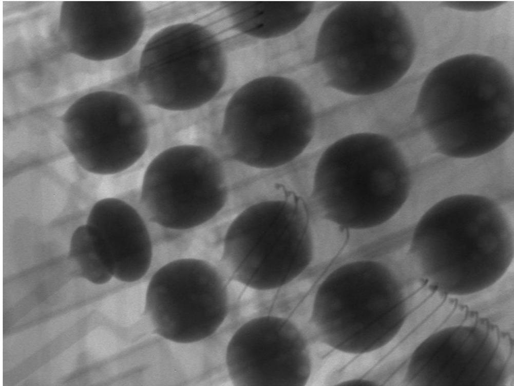
**Figure 1- HIP Defect in Corner of BGA**
