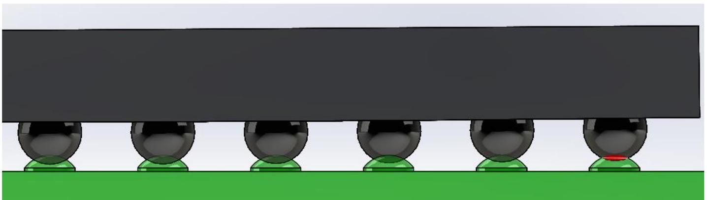
**Figure 6- Modeled View of BGA Ball to Solder Bump Contact with Original Stencil**
