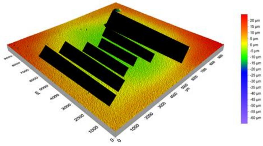
**Figure 4- Warp of Component As Delivered**
