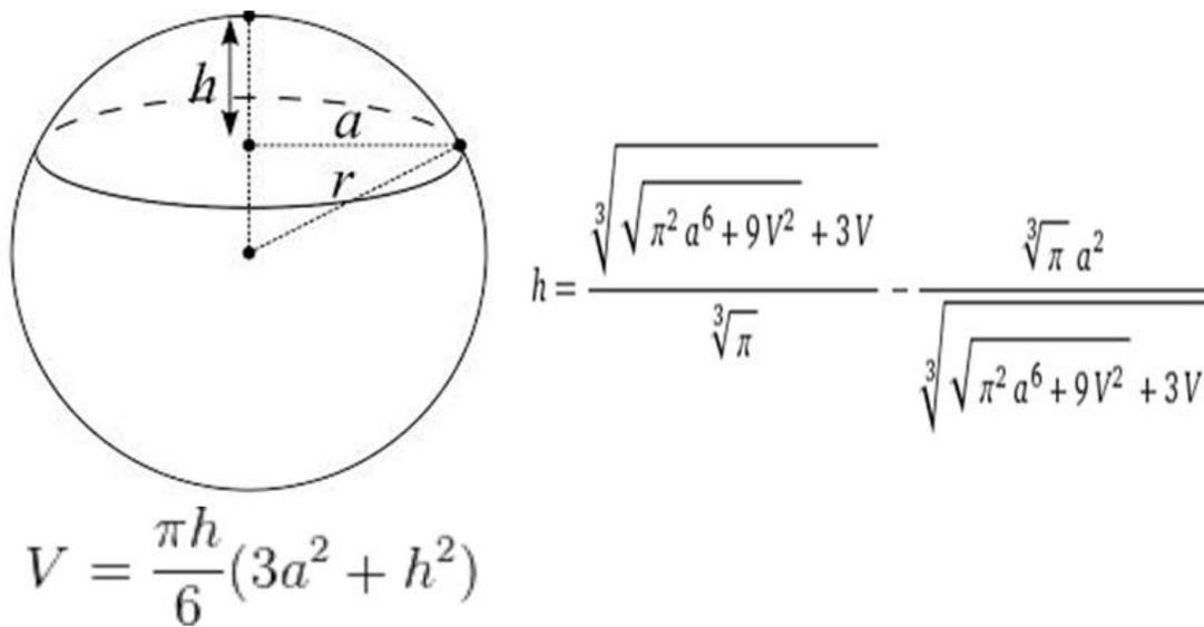
**Figure 7- Calculating Bump Height**
