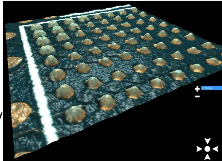
SPI view of paste deposits, showing lower transfer efficiency in center (right side in picture)
