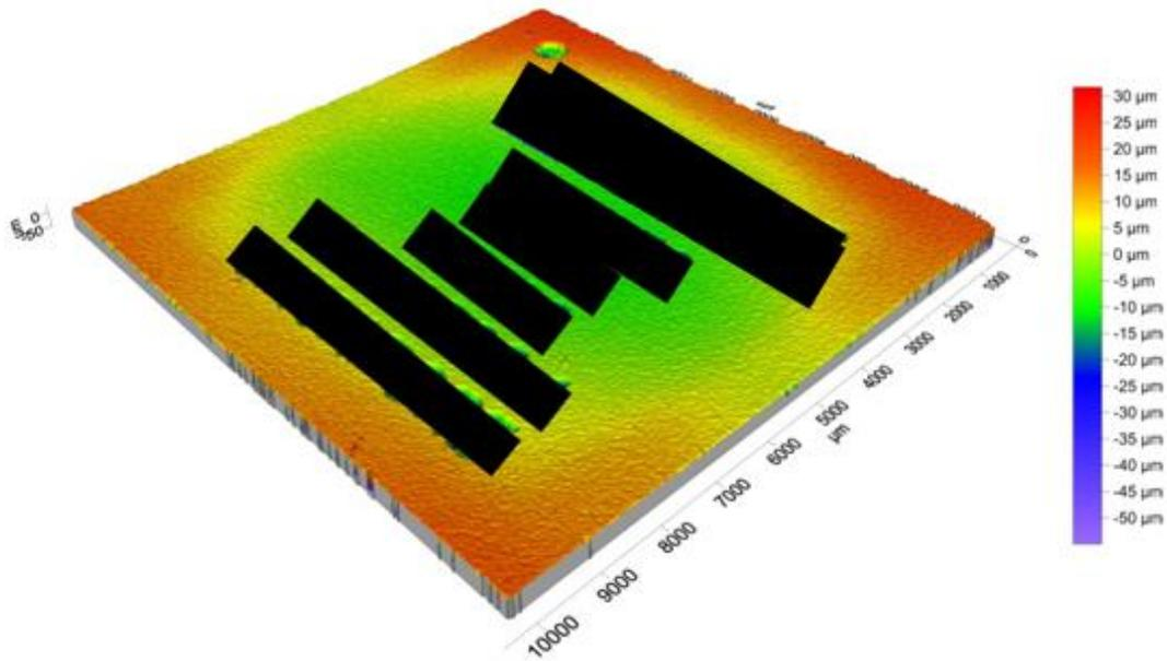
**Figure 5- Warp of Component After Soldering**
