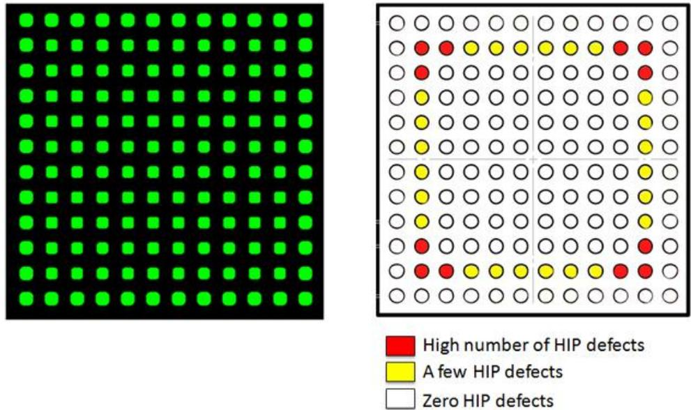
**Figure 3- Revised Stencil Design (left) and resulting shift in HIP defect location (right)**
