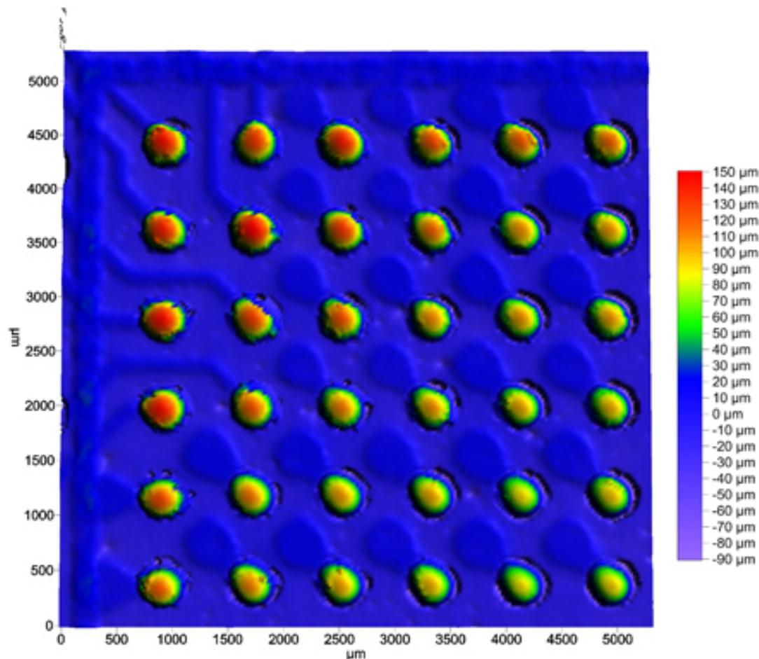
Scan of soldered bumps on bare board
