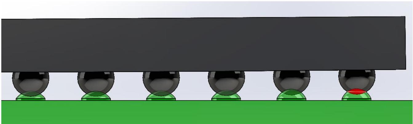
**Figure 10- Modeled View of BGA Ball to Solder Bump Contact with Variable Aperture Stencil**
