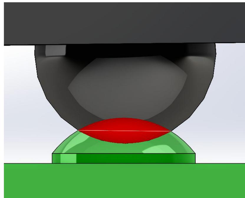
Model of solder ball in contact with molten bump. Interference area in red
