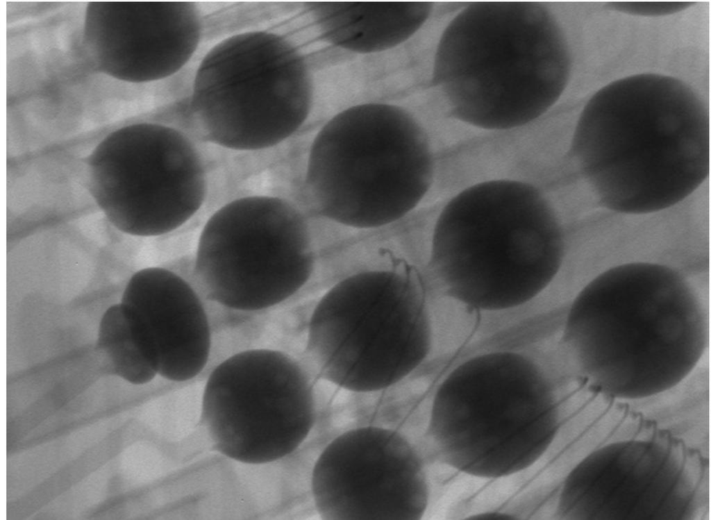
X-ray image showing HIP defect in production.
