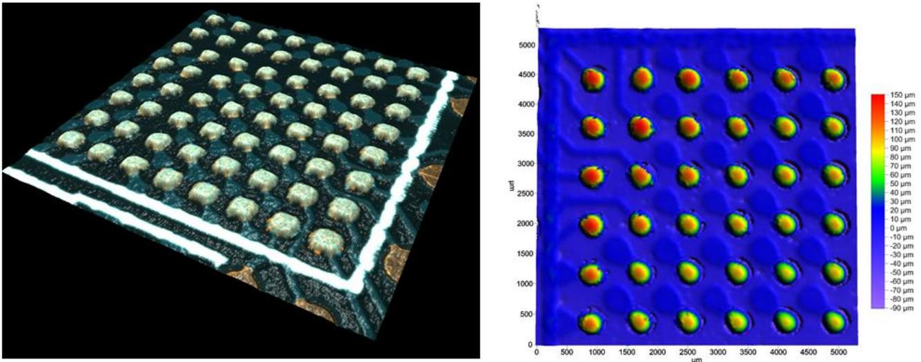
Figure 11- SPI Scan (left) and Bump Height Scan (right)
