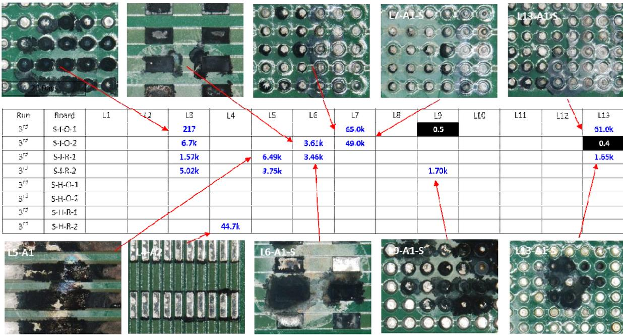
Figure 10: Company C 3<sup>rd</sup> run. Creep corrosion and resulting electrical shorts.
