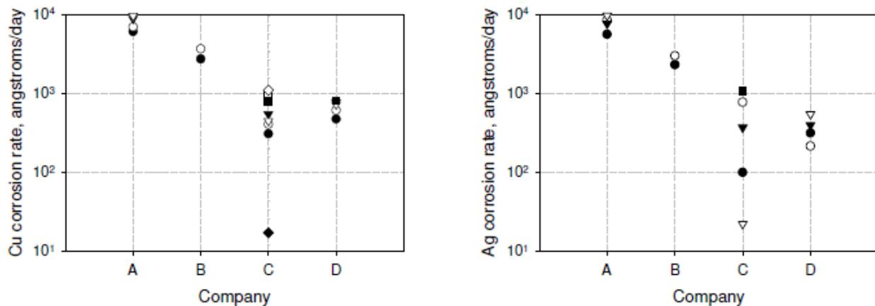
**Figure 4: Copper and silver corrosion rates in the first test run at the four companies.**
