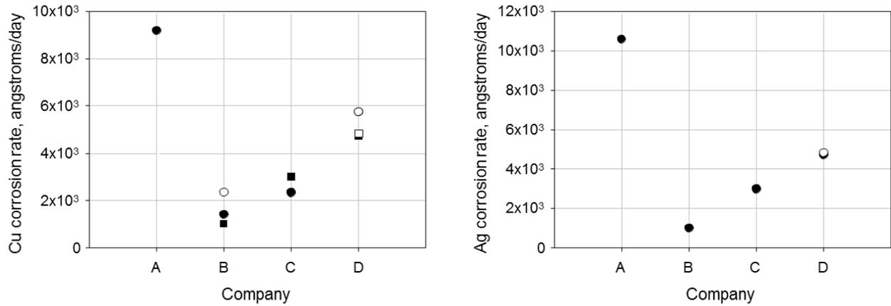
Figure 7: Copper and silver corrosion rates in the second test run at the four companies.
