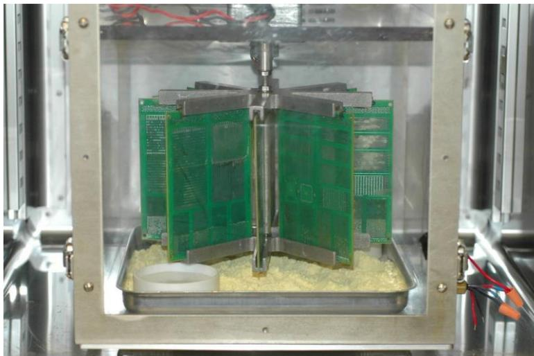
**Figure 6: Setup with increased area of sulfur bed used in the 2<sup>nd</sup> run.**
