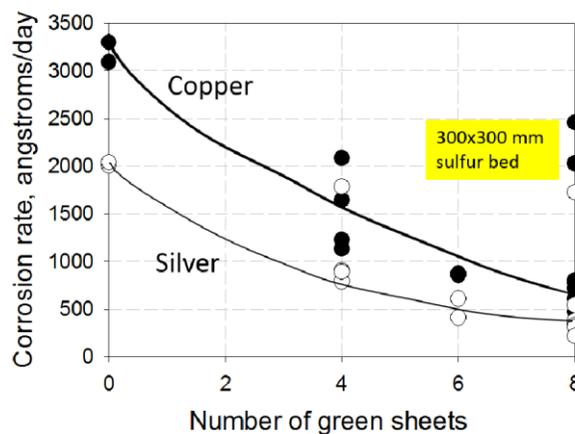
**Figure 3: Copper and silver corrosion rates as a function of PCB loading. The total number of boards, the sum of the brown epoxy boards and the PCBs (green sheets) was 8 in each of the runs.**
