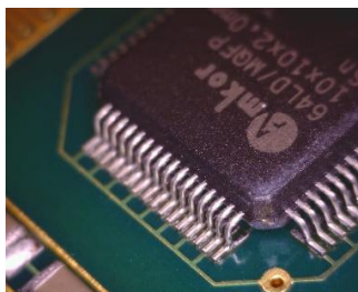
Fig 4. QFP leads at alternating polarity.
