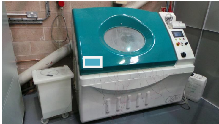
Fig 10. Humidity / Salt-mist chamber
