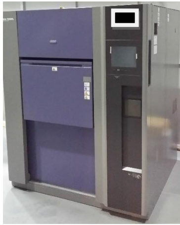
Fig 9. Production thermal shock chamber
