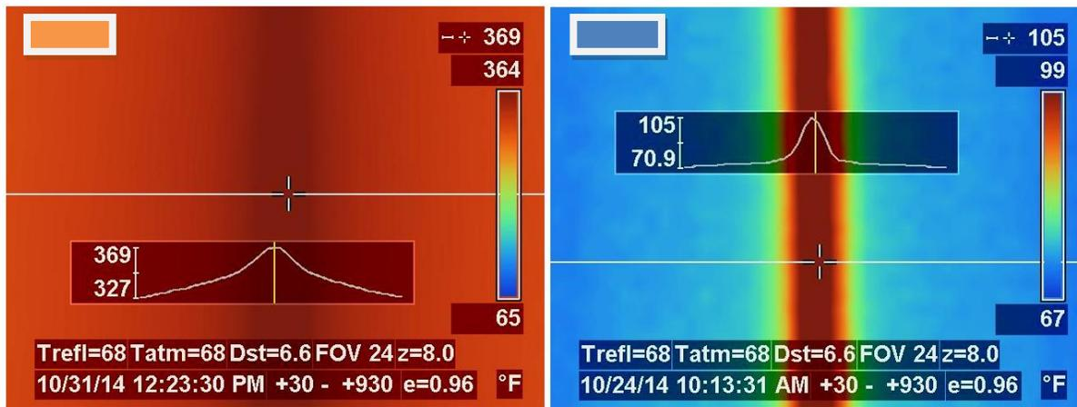
**Figure 7. Comparison of the same circuit without a heat sink attached on left and with a heat sink attached on the right picture. Both pictures are the top view and zoomed in for magnification of the conductor width which is about 21mils wide.**
