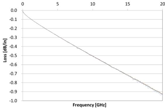
Figure 4(a). Extracted S21 thru two-line method over length difference with fixed L2.
