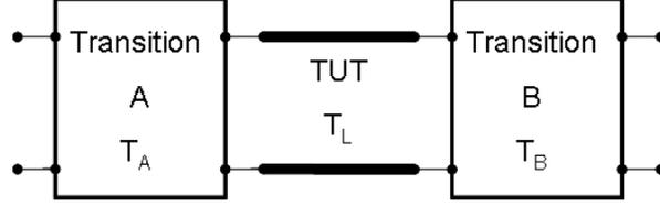
Figure 1. Connection diagram and associated cascade matrices for test line measurement. TUT represents transmission line under test.
