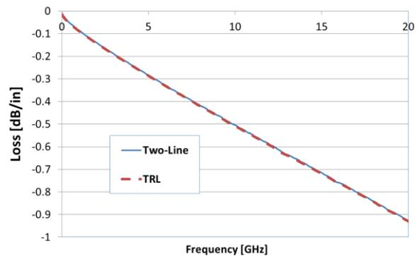
Figure 3(b). Comparison of recovered insertion loss of two-line and TRL method.
