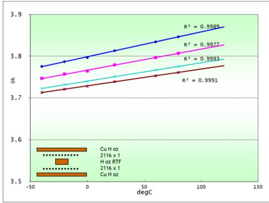
Figure 5(a). Extracted Dk over temperature and frequency at 4, 8, 15 and 20 GHz lines from up to down.
