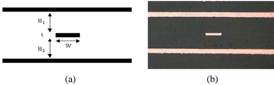
Figure 2. Pictorial structure diagram and associated parameters of a PCB stripline. (b) A real cross-section of a stripline embedded in PCB board.
