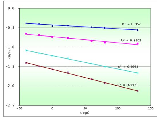
Figure 5(b). Extracted insertion loss over temperature and frequency at 4, 8, 15 and 20 GHz lines from up to down.
