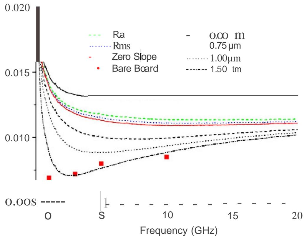
Simulation of dispersive  $\tan \delta$  based on different roughness or conductor-loss assumption.
