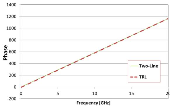
Figure 3(a). Comparison of recovered phase of two-line and TRL method.
