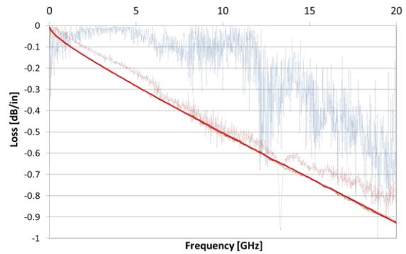
Figure 4(b). Extracted S21 thru two-line method over length difference with fixed L1.
