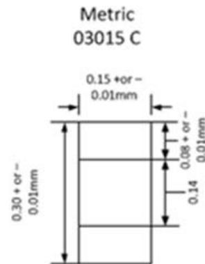
Show small gap placement without paste squeeze out shorting.
