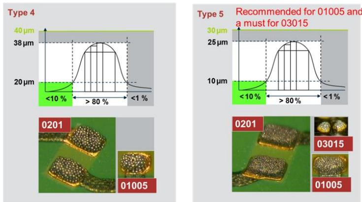
Fig. 8: Comparison of solder paste Type 4 and Type 5
