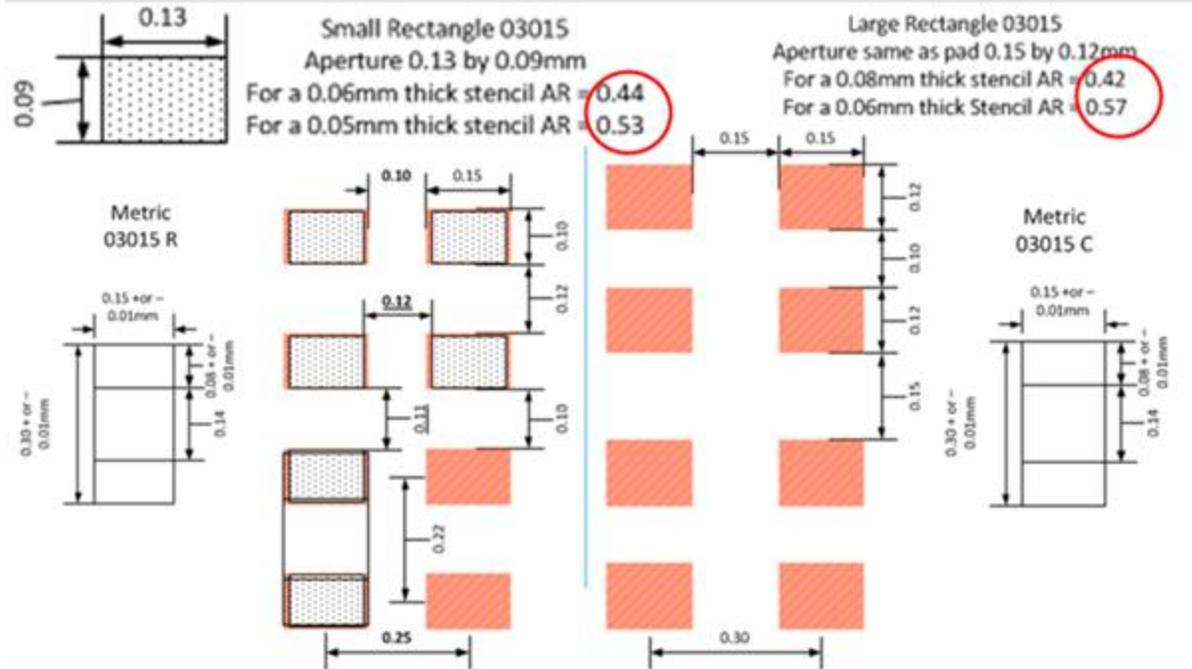
Fig. 1: Pad design: The smallest pad-aperture design gives an area ratio of 0.53
