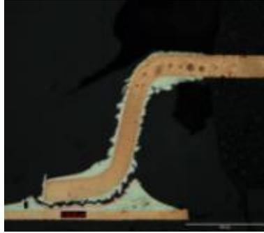
**Figure 8 – Cross section image of a solder joint after TCoB testing.**
