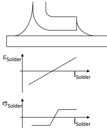
**Figure 4 – Schematic tensile deformation in a gull wing lead solder joint and stress distribution at the end of a temperature dwell**
