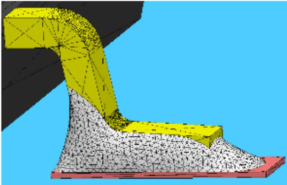
*a) Reference solder joint (100% solder volume)*
