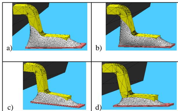
**Figure 7 – Different solder joint shapes. a) 100% solder volume, b) 120% solder volume, c) 80% solder volume, d) 50% solder volume**
