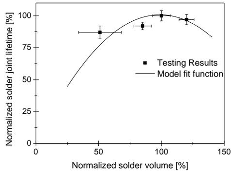
**Figure 6 – Solder joint lifetime as a function of solder volume**
