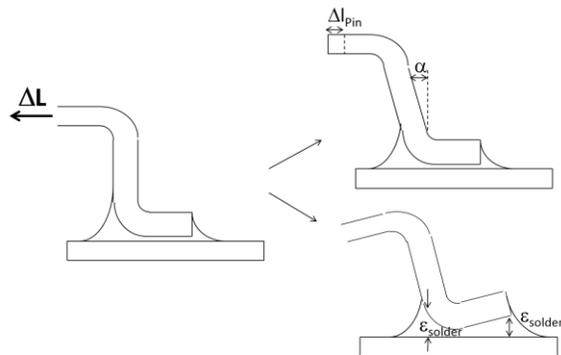
**Figure 3 – Deformation of pin and solder joint due to CTE-mismatch of component and PCB**
