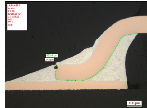
*SOT23 pins with different amounts of solder volume*
