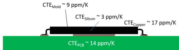
**Figure 2 – Schematic drawing of Quad Flat Package soldered on a PCB**
